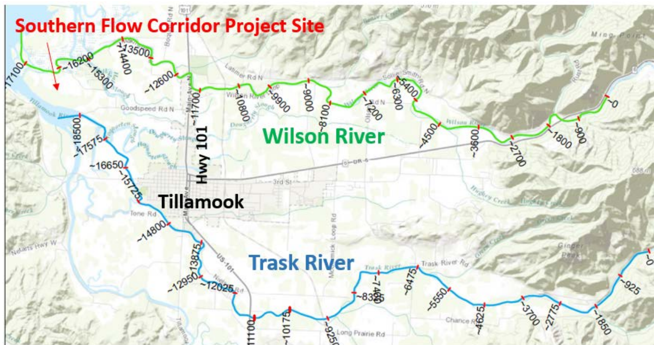
Figure 9. Approximate Stationing Along the Wilson and Trask Rivers in HEC-RAS Model.
