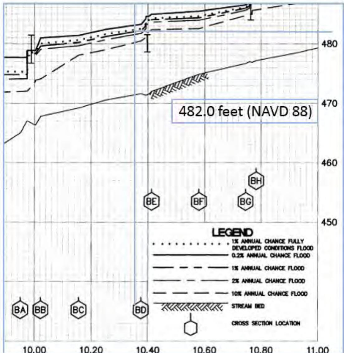
Figure 9: Portion of Stream Profile Used to Obtain BFE
