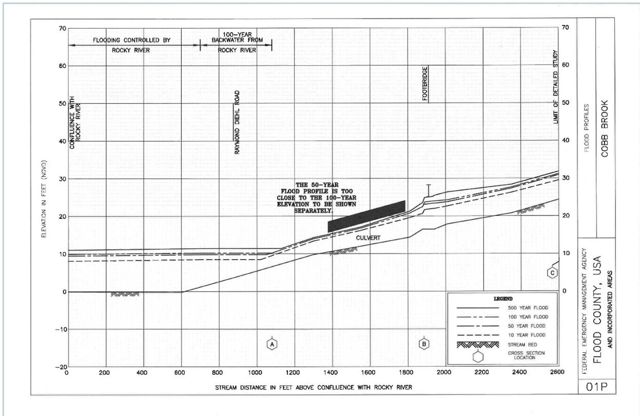
**Figure 7: Example of Stream Profile from FIS Report**
