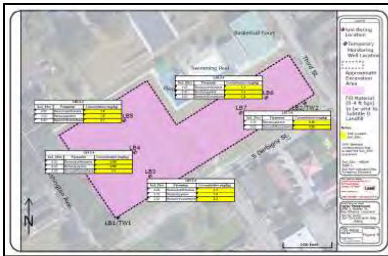
Figure 37. Taylor Playground Leaf Environmental, LLC Soil Borings and Results. Pink area is the excavation area which COC exceeds standards and must be disposed of at a Subtitle D Landfill.
