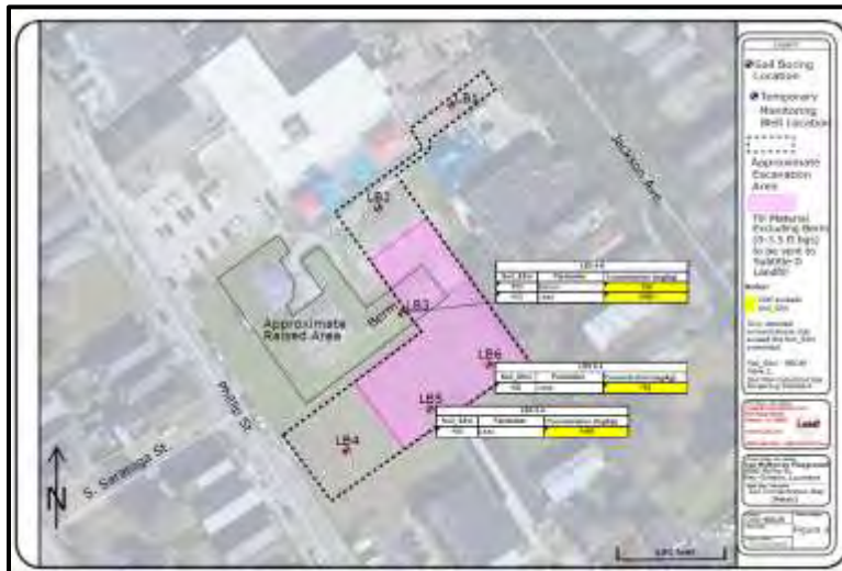
Figure 39. Van McMurray Leaa Environmental, LLC Soil Borings and Results for RCRA Metals. Pink area is the excavation area which COC exceeds standards and must be disposed of at a Subtitle D Landfill
