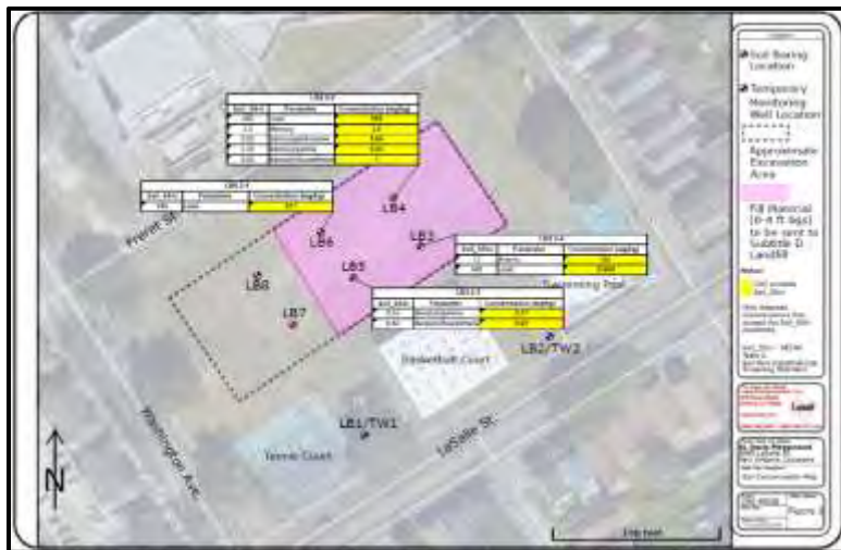
Figure 30. A.L. Davis Park Leaf Environmental, LLC Soil Borings and Results. Pink area is the excavation area which COC exceeds standards and must be disposed of at a Subtitle D Landfill
