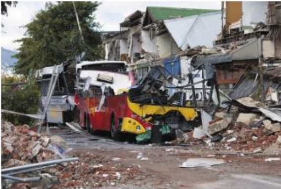
Figure 1. City bus crushed by URM debris falling from nearby buildings during the 2011 Christchurch earthquake in New Zealand. Twelve of the 13 people on board were killed. Photo credit: Simon Baker6.
