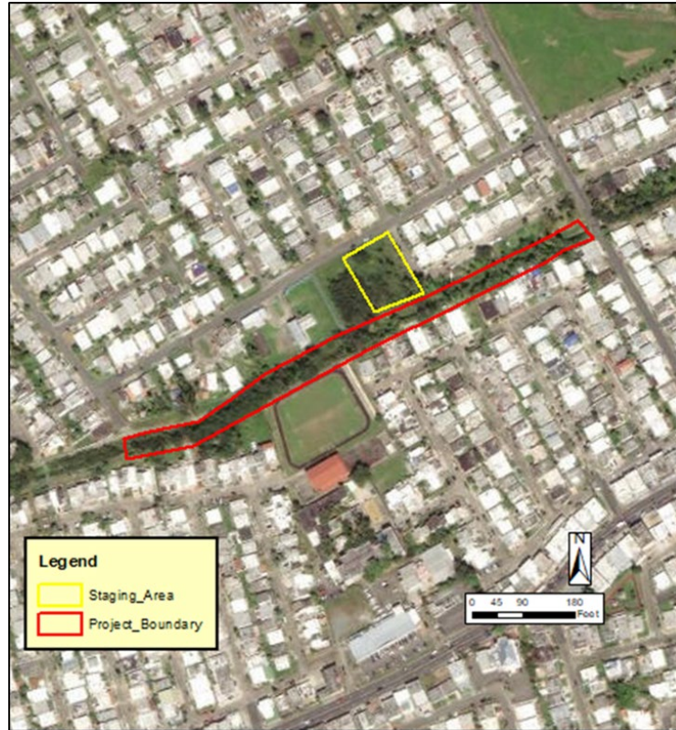
Figure 1. Example of a project site map for a streambank stabilization project. The map identifies the project boundaries and staging area and includes a north arrow and a scale.
