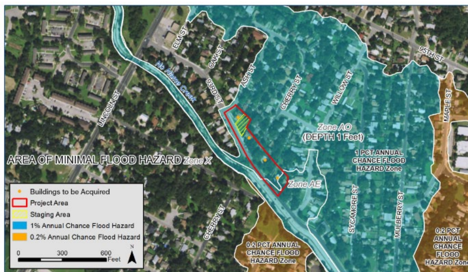
Figure 3. Example of a project site map. Map clearly shows the buildings to be acquired, the project area, the staging area, the flood zones and flood source and the base flood elevation for the project site. The map includes a north arrow and a scale.
