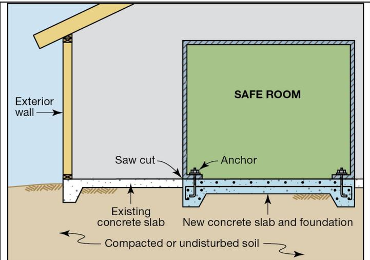
**Figure 2: New concrete slab foundation that has been designed to meet the requirements of FEMA P-361 and ICC 500 Section 307**
