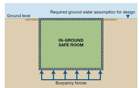
**Figure 3: Ground water level for in-ground safe room**
