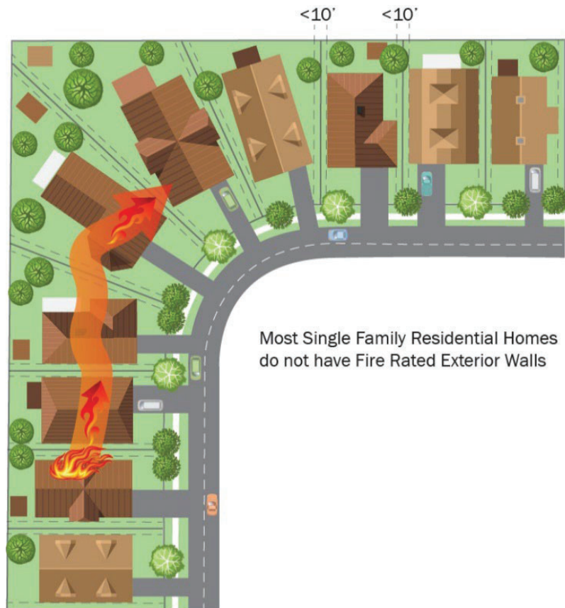
Figure 2. Typical residential building separations (10–20 feet) are vulnerable to structure-to-structure fire spread under extreme wildfire conditions, as most single-family residences have non-fire rated exterior walls.
