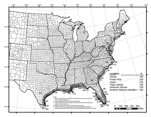
Figure 2: Design wind speeds for hurricane storm shelters
