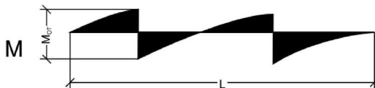
Figure 5-32 Moment distribution in the concrete grade beam.
