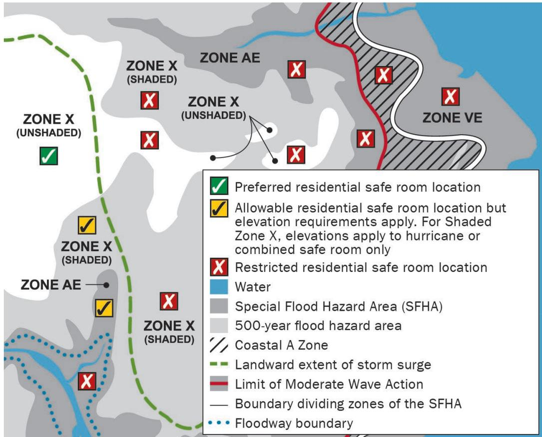
**Figure B4-4: Example illustration of preferred, allowable, and restricted residential safe room locations**
