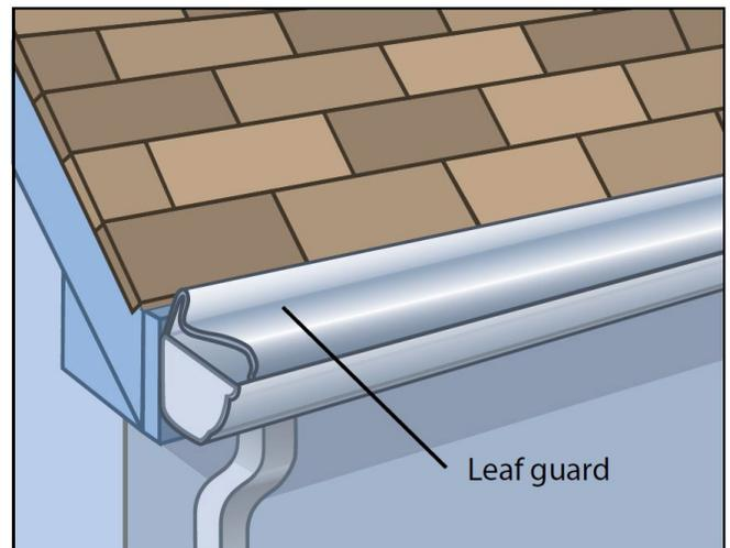
**Figure 2. Leaf guards allow rainwater into the gutter but keep combustible debris out.**
