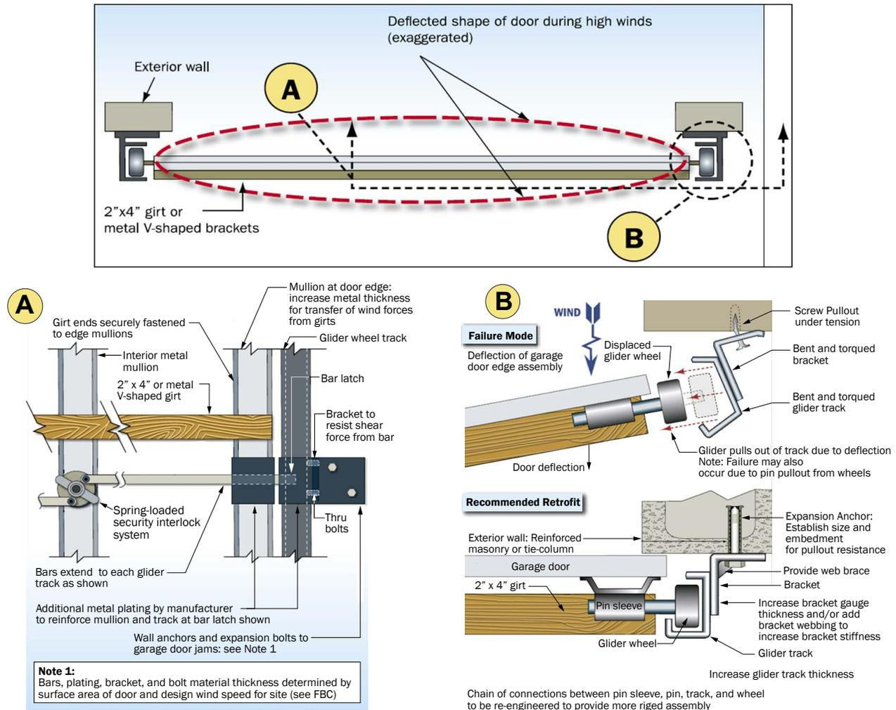
**Figure 3.2.5. Recommended details for upgrading garage doors.**
