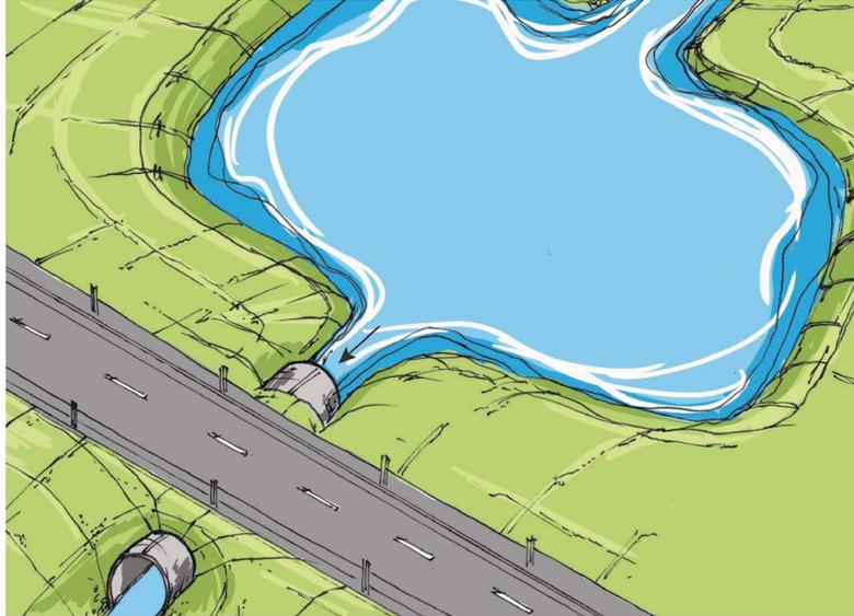
**Figure 1.3.19. A sediment basin can help settle suspended sediment and decrease culvert clogging potential.**
