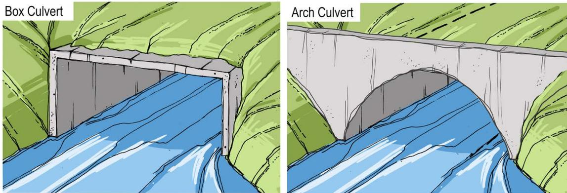
Figure 1.3.4. An arch culvert or a box culvert can provide increased flow capacity.
