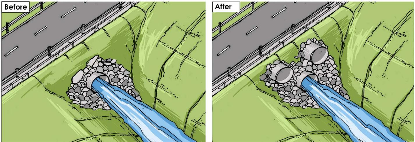
**Figure 1.3.6. Installing multiple culverts can increase flow capacity.**
