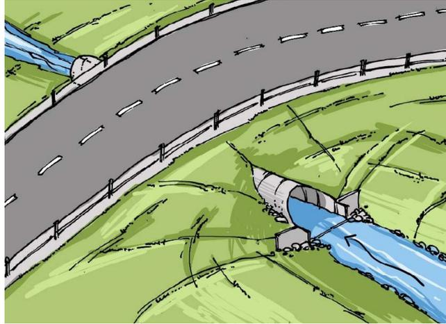
**Figure 1.3.8. A cutoff wall can reduce undermining.**
