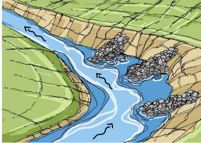
Figure 1.3.15. Flow diverters can realign the stream channel.
