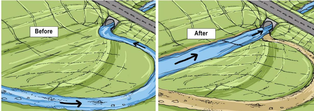
Figure 1.3.17. Realigning the stream can protect embankments.
