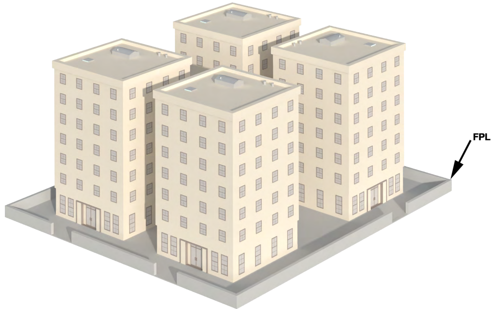
Figure 5-6. Example of perimeter floodwall around multi-family buildings (Note temporary shields are required for the openings)
