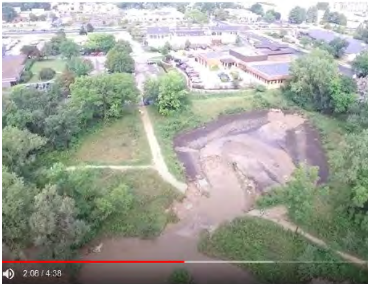
Photo 48: Site 36 (August 2018), provided by the applicant. Taken at 43.10524, -89.50864. Donna Pond. View of collapsed embankment.
