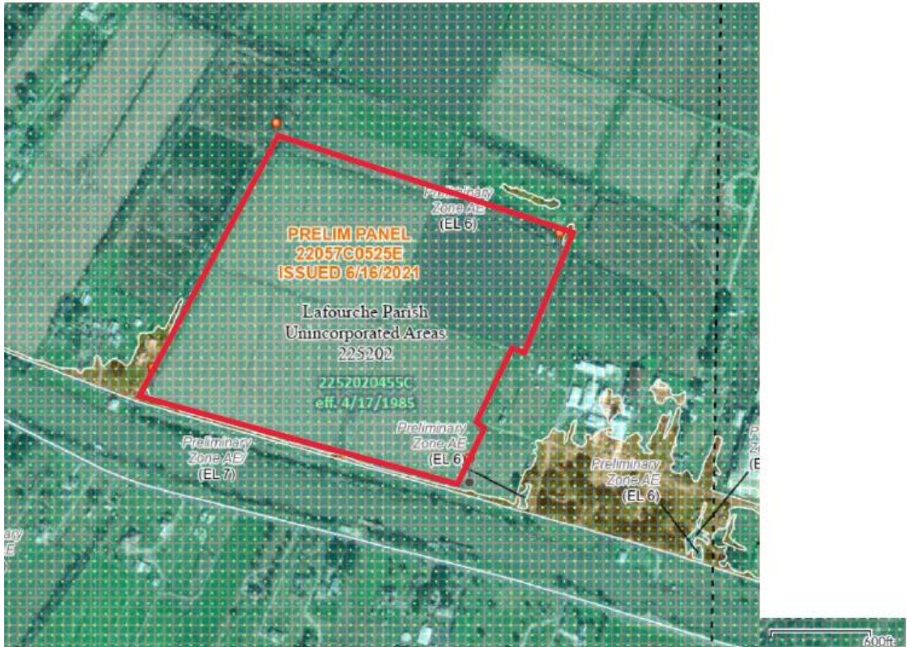
Figure 3: Flood Insurance Rate Map (FIRM) for the Proposed Valentine #3 Subset Group Site
