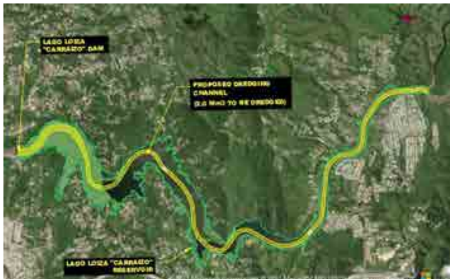
Figure 2. Conceptual design of dredging channel, courtesy of Puerto Rico Aqueduct and Sewer Authority
