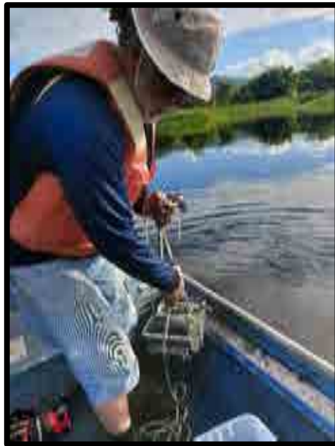
Figure 2. Petite Ponar Dredge sediment sampling equipment used in Carraizo Peservoir
