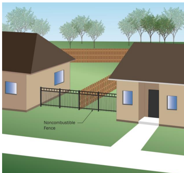
Figure 6. Noncombustible materials should be used to construct at least the first 5 feet of a fence attaching to a home.
