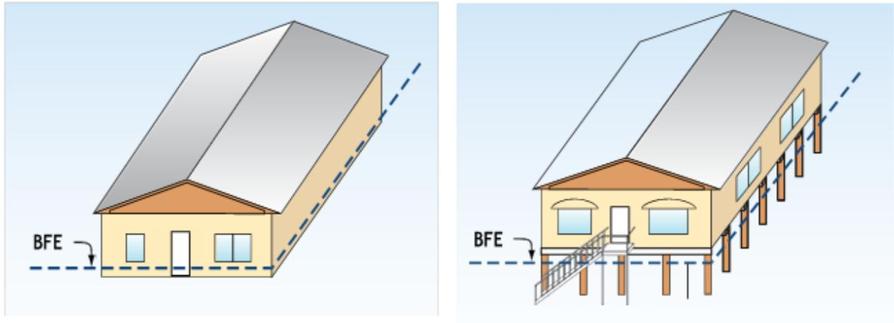
**Figure 1: Elevating a house above the Base Flood Elevation can mitigate future flood damage**
