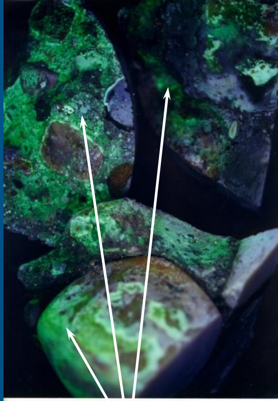
ASR affected concrete/aggregate observed during a petrographic examination.
