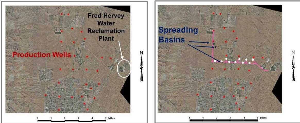
Figure 3-7. Injection Wells and Spreading Basins Interspersed in El Paso, Texas Water Supply Well field
