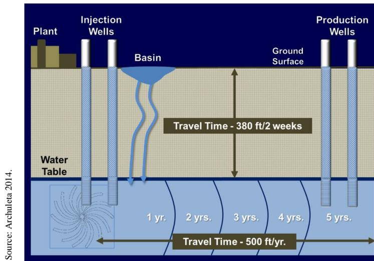
Figure 3-4. Typical ARAR System Operation
