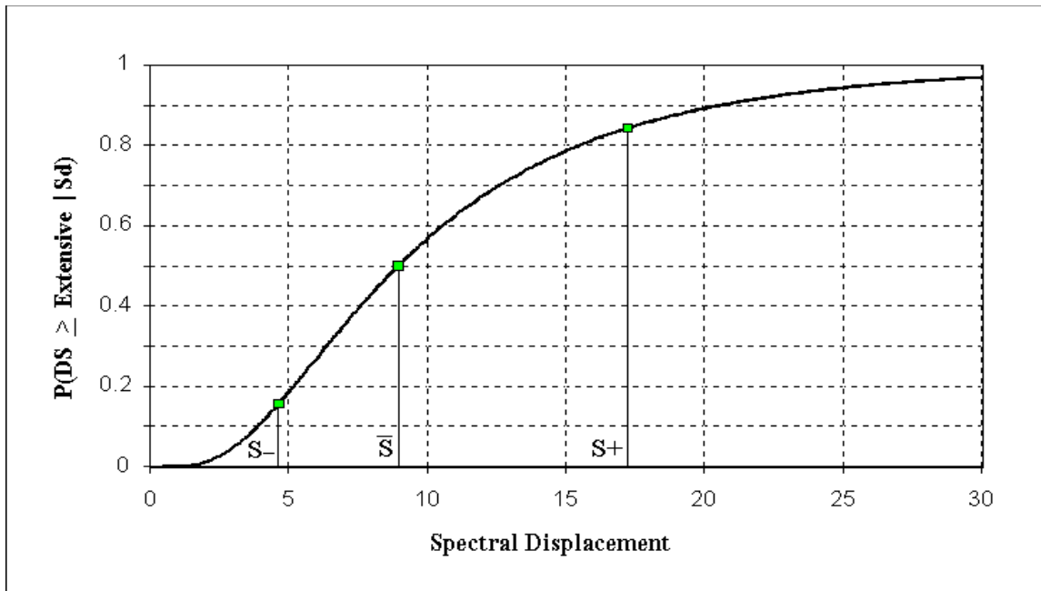
Figure 5-5 Example Fragility Curve - Extensive Structural Damage, C1M Specific Building Type, High-Code Seismic Design
