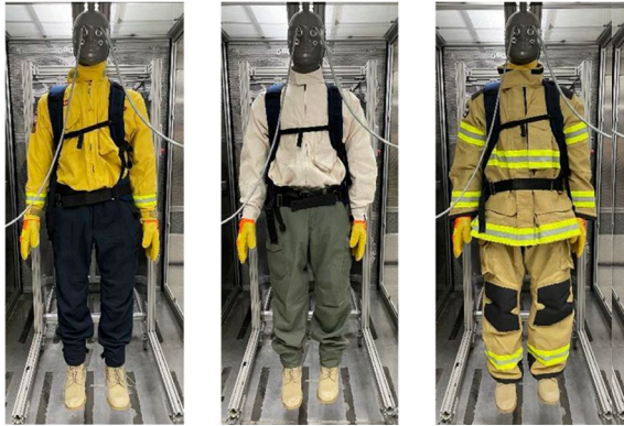
Figure 5. Wildland / WUI ensembles evaluated using sweating manikins: NFPA 1977 wildland ensemble (left), particle blocking (middle), and standard turnout outer shell (right).
