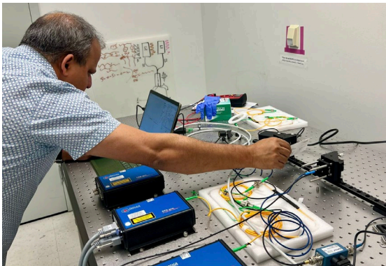
Figure 4. Terahertz laser set-up with mixtures of aerosols being recorded in the presence and absence of object interference.
