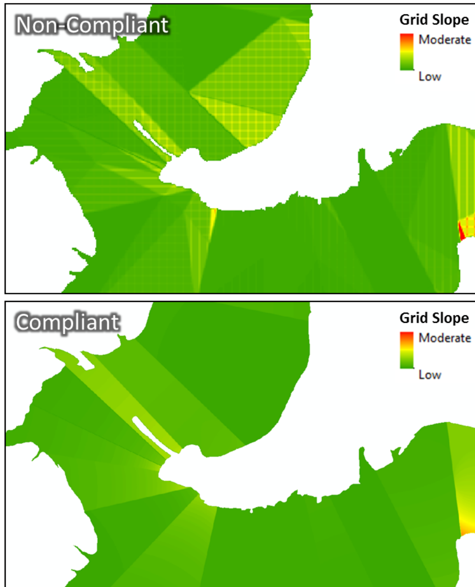
Figure 15: Slope Raster Reveals WSEL Raster Anomalies in Between Cross-Sections
