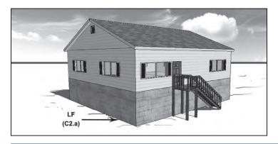
**Building Description** 1 floor with finished or unfinished enclosed area (see EC, Diagram 7)
