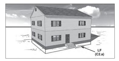
**Building Description** 2 floors with subgrade crawlspace with or without openings (see EC, Diagram 9)
