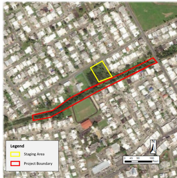
Figure 2. Example of a project site map. Map clearly shows the project area boundary and the staging areas. The site features are overlaid on an aerial photo and include a north arrow and a scale.
