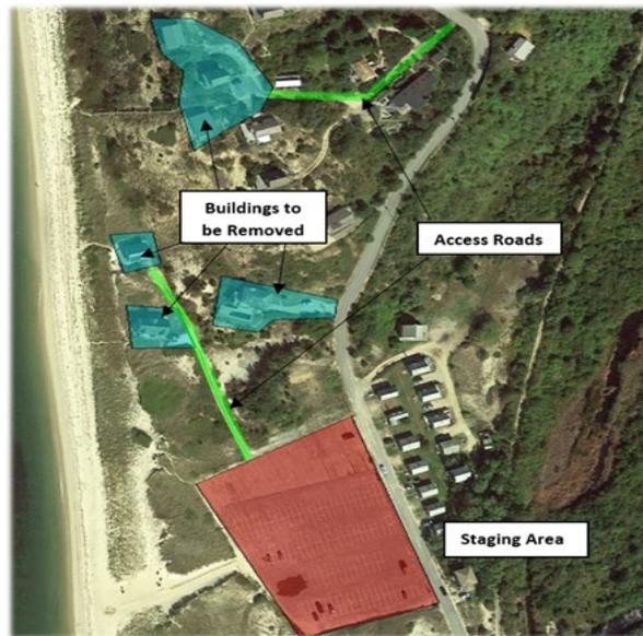
**Figure 2. An example of a project site map. Map clearly shows the buildings to be demolished, the staging area and the access route into the work area. The site features are overlaid on an aerial photo.**
