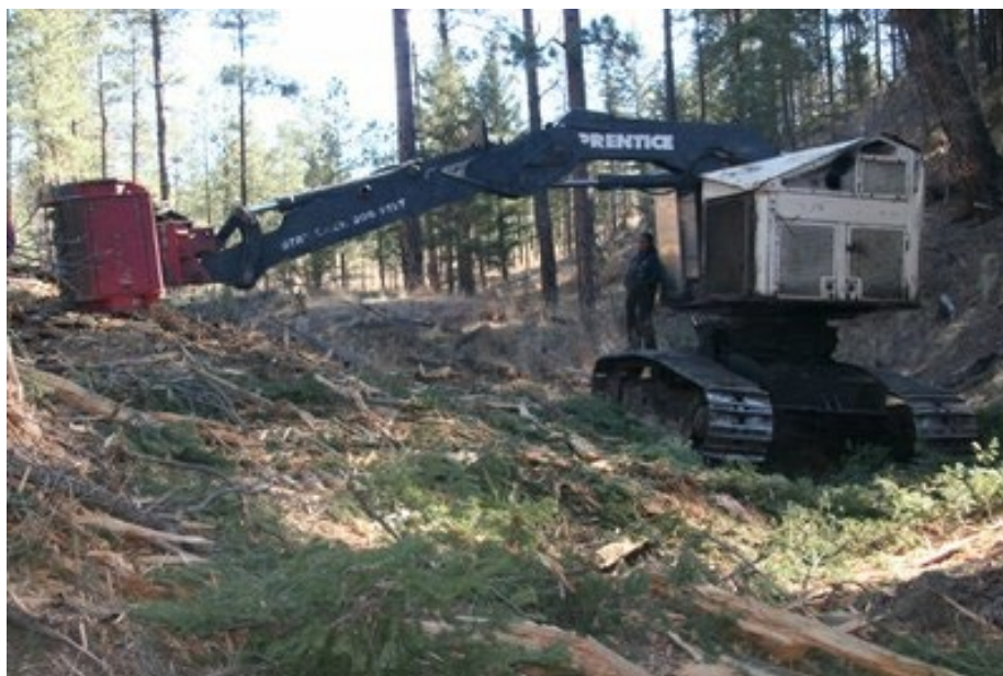
6. Hillslope Cover Application: Slash spreading mechanical equipment
