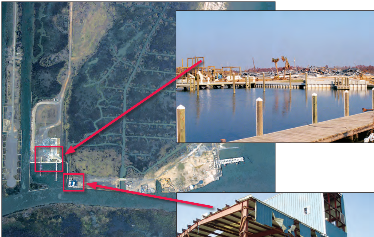
Figure 3-21. A reinforced concrete and pre-engineered metal building (PEMB) housing a seafood processing building sustained severe damage due to storm surge, waves, and floating debris. Nearby marina buildings were also destroyed (Lakeshore area, Hancock County, Mississippi).
