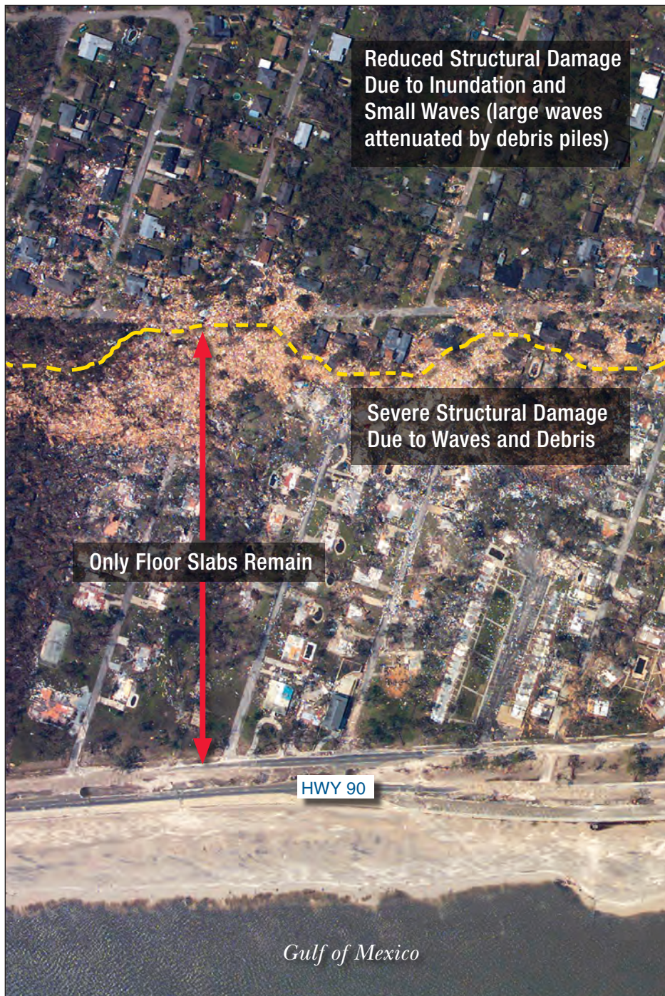
Figure 4-38. Typical zones of damage to homes supported on slab-on-grade foundations (Pass Christian, Mississippi)
