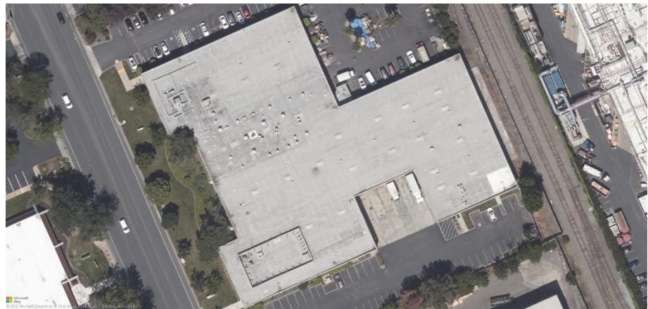
Figure 8-1      Example of a RWFD building with a large re-entrant corner
