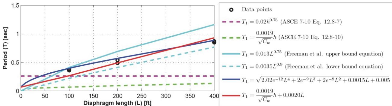
Figure B-6 Comparison of fundamental periods from analyses of wood panel archetypes to those predicted by the proposed formula (Equation B-1), ASCE/SEI 7-10 equations, a best fit curve, and those proposed by Freeman et al. (1995).
