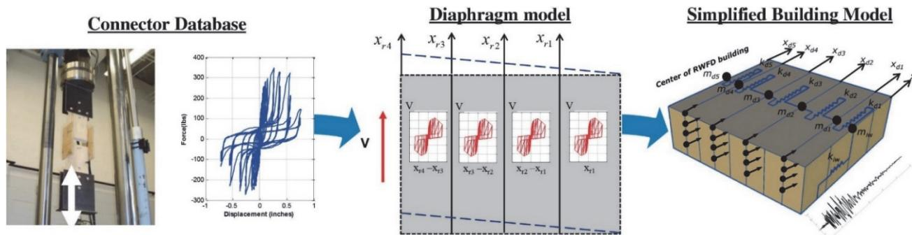
Figure A-1 Three-step modeling framework.
