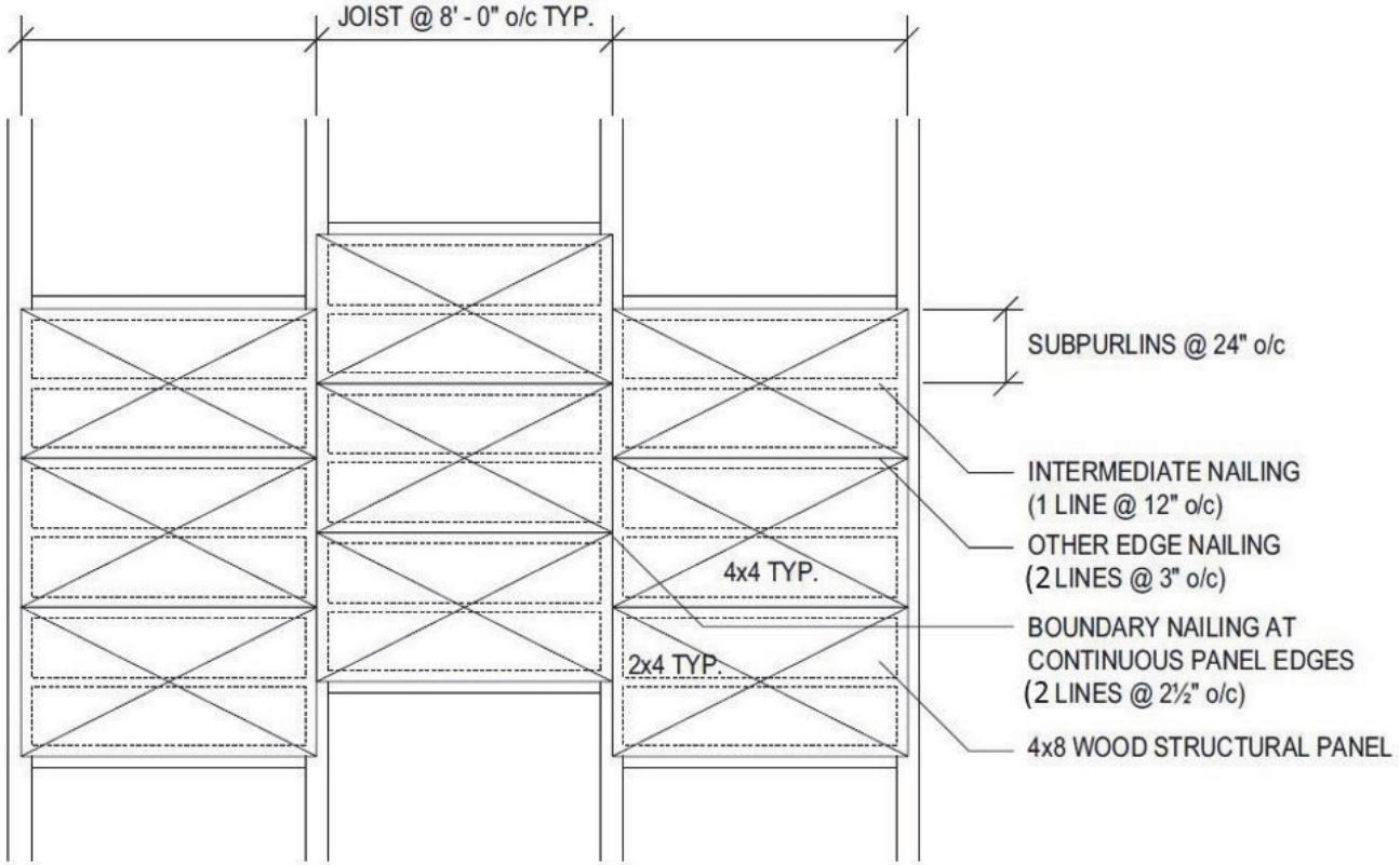
Figure 3-4 Sheathing layout and nailing for a panelized roof system (Lawson, 2013).
