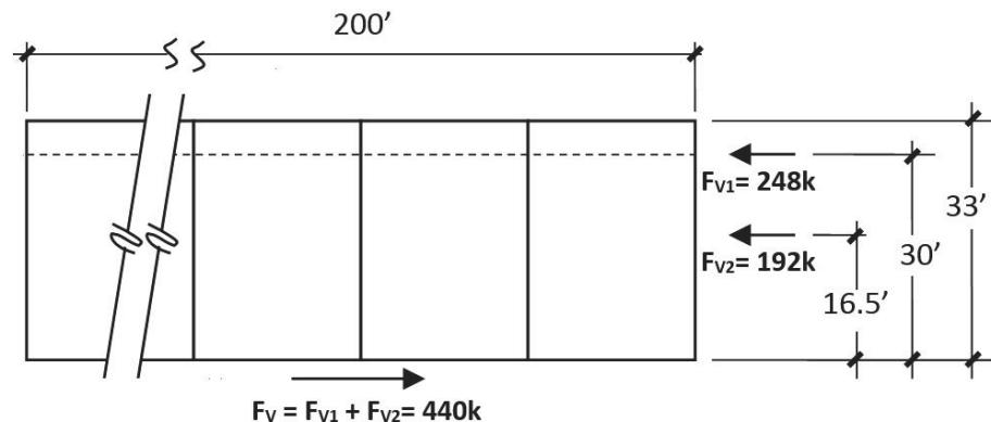
Figure 5-6      North/south lateral design forces acting on the shear walls (Lines A & J).
