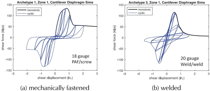
Figure D-5 Response in cantilever diaphragm simulation comparing the roof zone closest to the edge of the building for roof that is: (a) mechanically fastened, and (b) welded (figure credit: Schafer, 2019).
