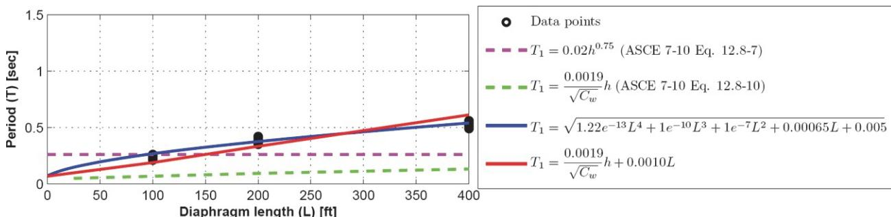
Figure B-7 Comparison of fundamental periods from analyses of steel deck archetypes to those predicted by the proposed formula (Equation B-3), ASCE/SEI 7-10 equations, and a best fit curve.
