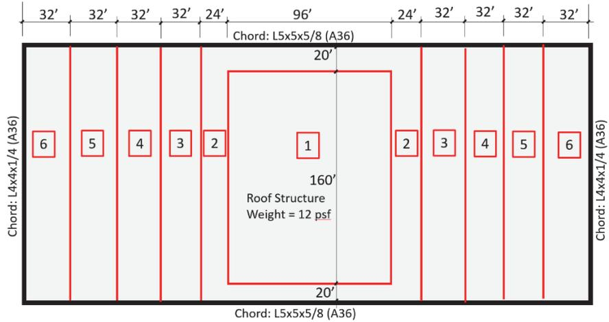
Figure B-2 Design details for the "large" archetypes with wood diaphragms designed for high-seismic hazard (traditional procedure).
