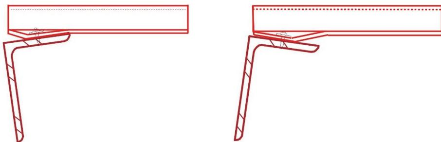
(b) Potential deck bending for roof drift to the left.
