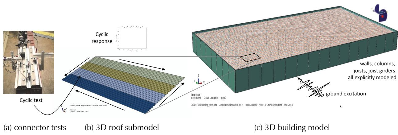
Figure D-4 3D building model employed in simulations (figure credit: Schafer, 2019).
