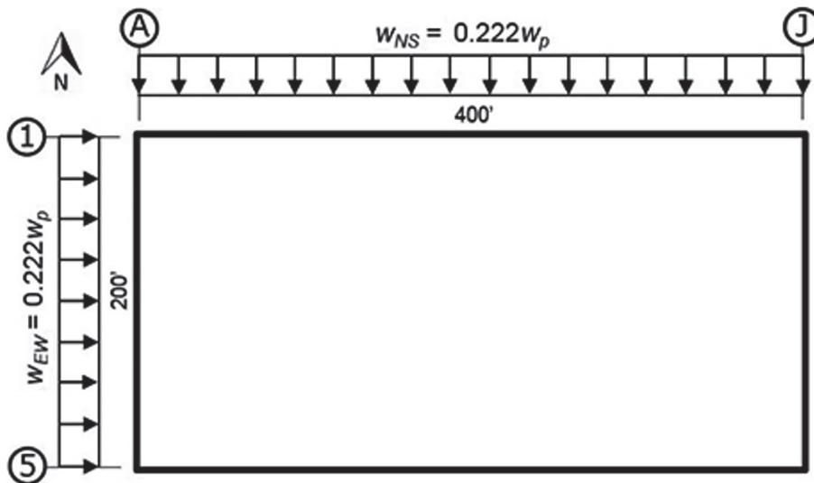
Figure 5-8 Diaphragm loading model (alternative RWFD procedure).
