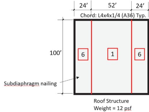
Figure B-3 Design details for the “small” archetypes with wood diaphragms designed for high-seismic hazard (traditional procedure).
