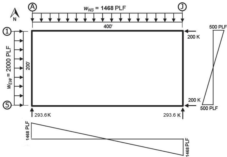
Figure 5-9 Diaphragm shear distribution.
