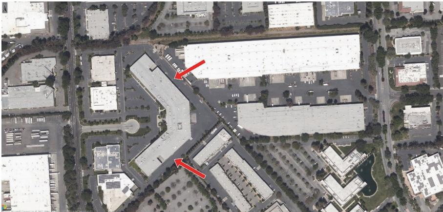
Figure 8-4 Example of a RWFD building with nonparallel walls (photo credit: ConnectExplorer).
