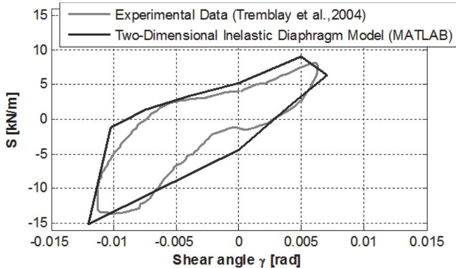
Figure A-8 Validation/comparison of inelastic roof diaphragm for cyclic loading (one main cycle).
