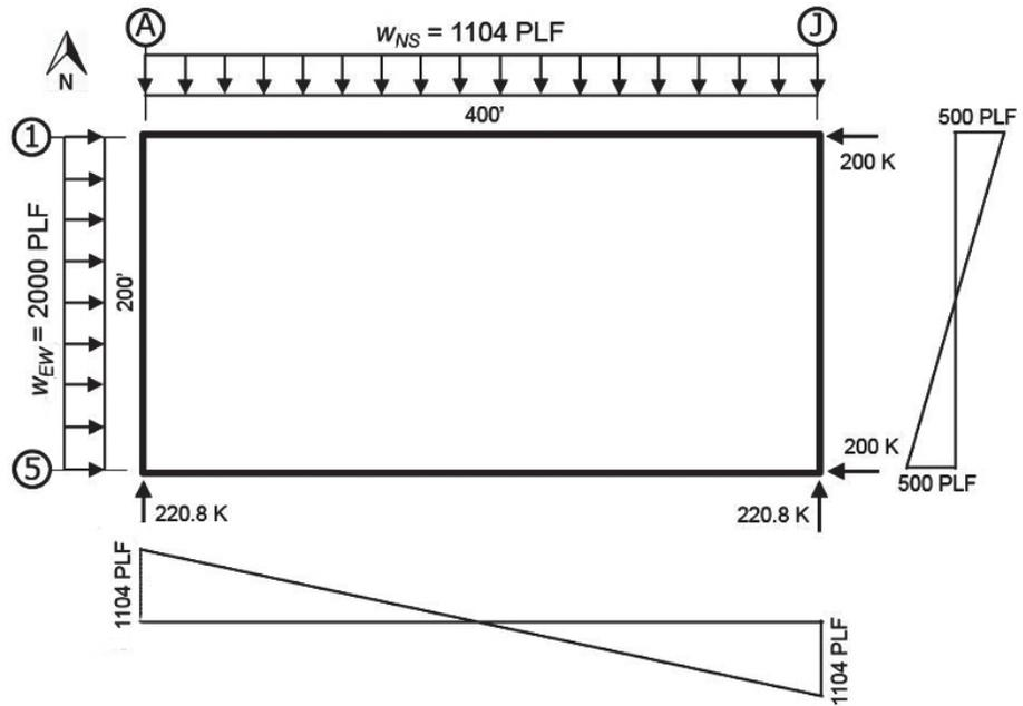
Figure 5-2 Diaphragm shear distribution.
