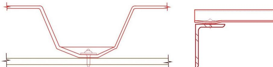
(d) Potential deck bending that reduces prying due to roof drift.
