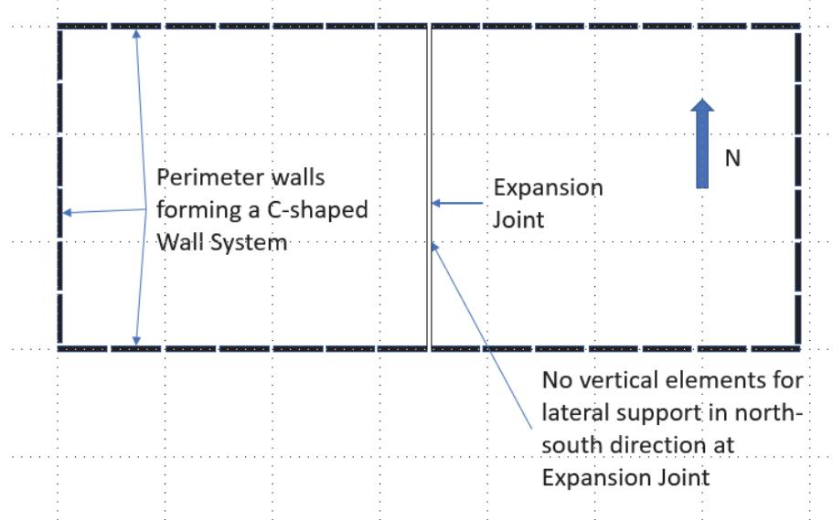
Figure 8-6 C-shaped lateral-system configuration.
