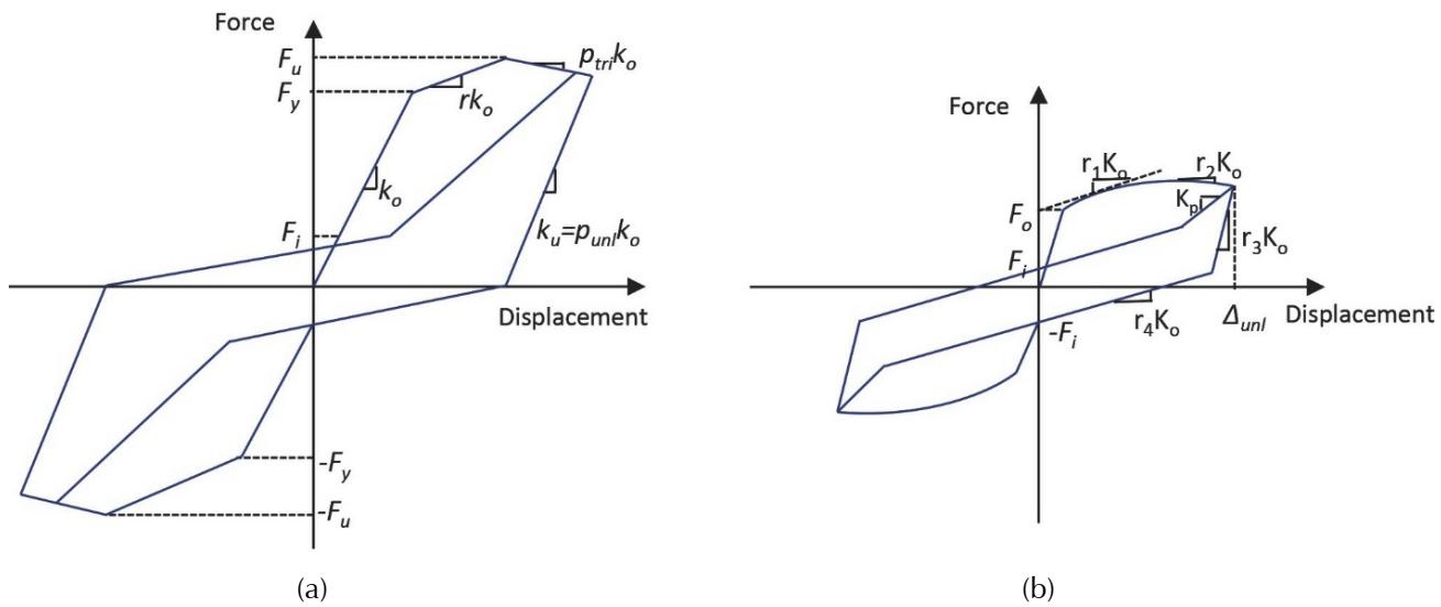
Figure A-2 Illustration of hysteretic models: (a) Wayne-Stewart; and (b) SAWS.
