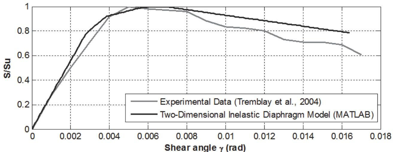
Figure A-7 Validation/comparison of inelastic roof diaphragm for monotonic loading.
