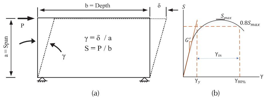
Figure D-3      Definition of: (a) shear angle ( $\gamma$ ) and normalized load ( $S$ ) in typical cantilever test, and (b) stiffness ( $G'$ ), strength ( $S_{max}$ ), and subassembly ductility ( $\mu_{sub}$ ) evaluated from test results (figure credits: (a) O'Brien et al., 2017; (b) Schafer, 2019).
