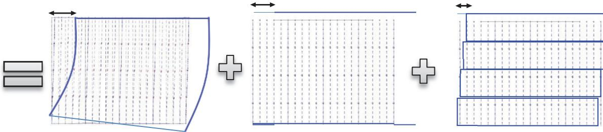
Figure A-5 In-plane displacement components of the analytical inelastic roof diaphragm model.
