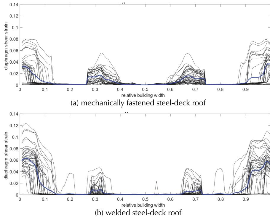
Figure D-7 Trace of peak mid-width diaphragm shear strain across 400-foot roof width for forty-four earthquake records with average in blue for: (a) mechanically fastened roof, and (b) welded roof.
