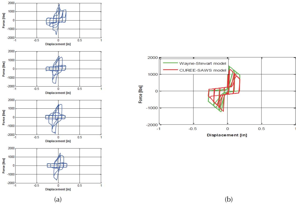
Figure A-4 Comparison of hysteretic response for 2-ply, 22-gage framing welds to 0.25 in. plate: (a) experimental (Guenfoud et al., 2010) and (b) fitted optimal hysteretic models.
