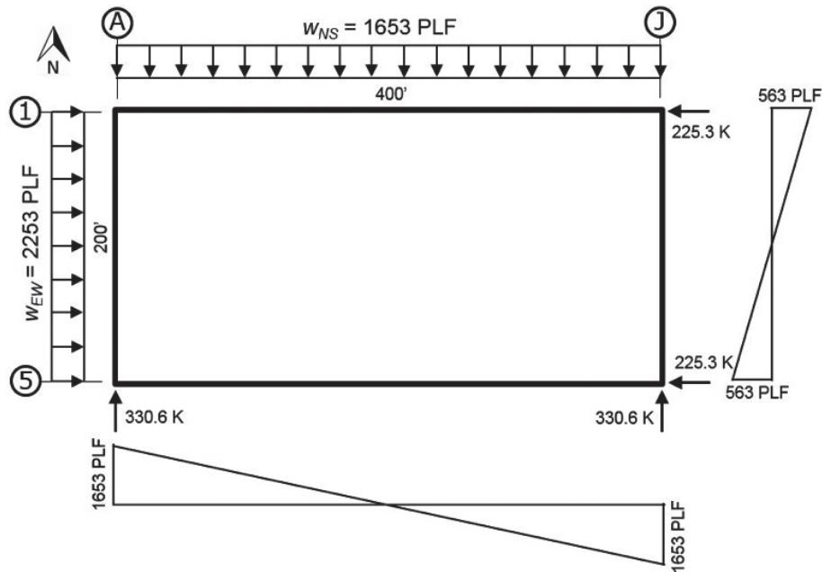
Figure 3-3 Diaphragm shear distribution in both orthogonal directions.
