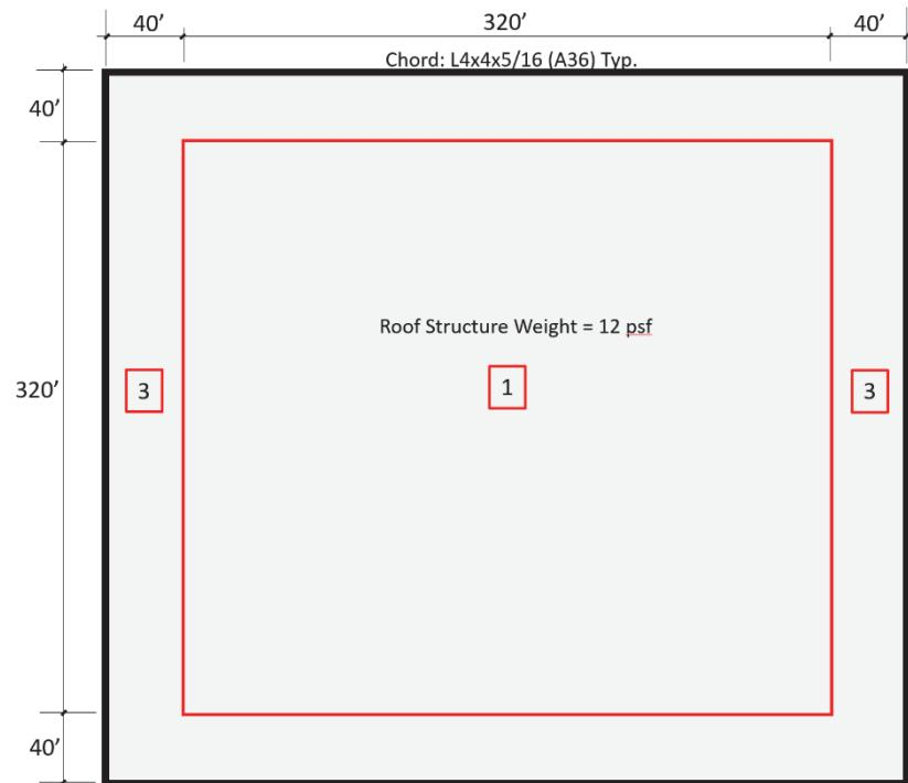
Figure C-1 Design details for archetypes with wood diaphragms designed for high-seismic hazard, part 1 (alternative RWFD procedure).
