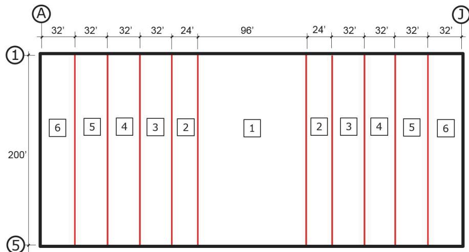
Figure 3-5 North/south nailing zone layout.
