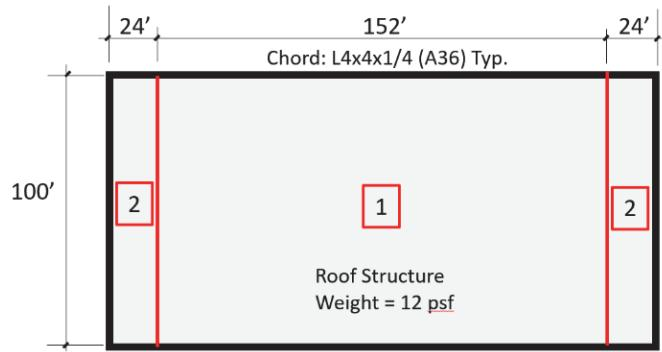
Figure B-5      Design details for "small" archetypes with wood diaphragms designed for moderate-seismic hazard (traditional procedure).
