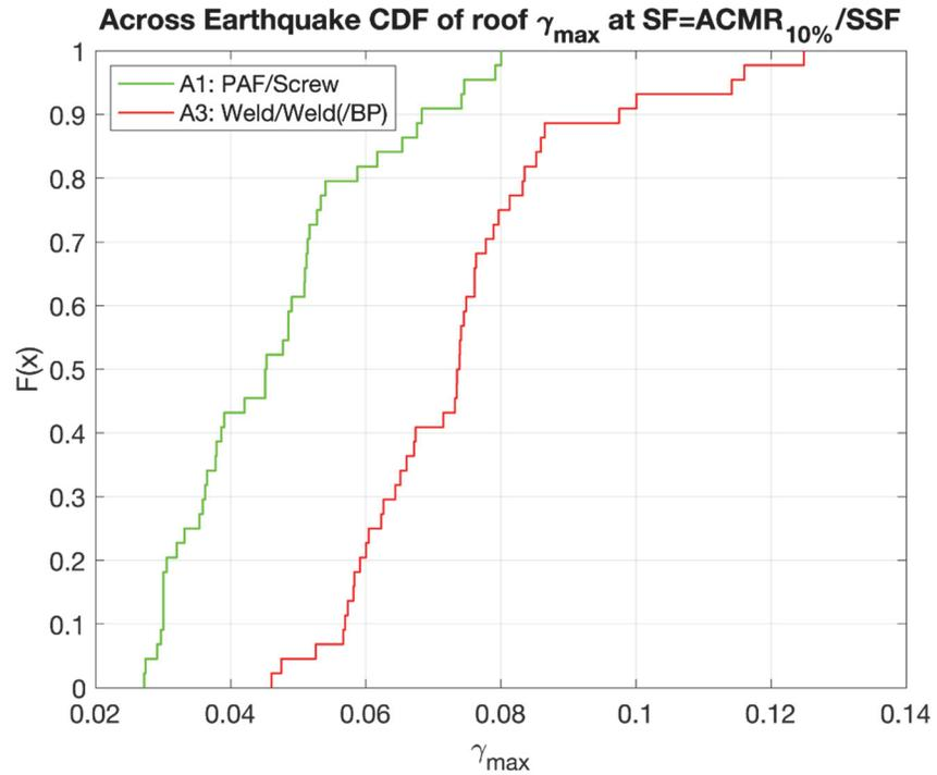
Figure D-6 CDF of peak diaphragm shear strain for large building archetype, mechanically fastened (designated as A1) and welded (designated as A3) across forty-four FEMA P695 earthquakes.
