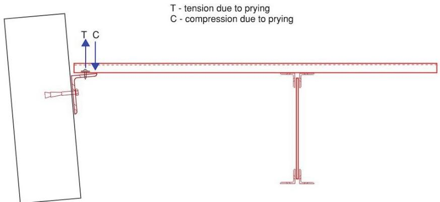
(a) Potential prying at deck-to-ledger angle caused by roof drift to the left.
