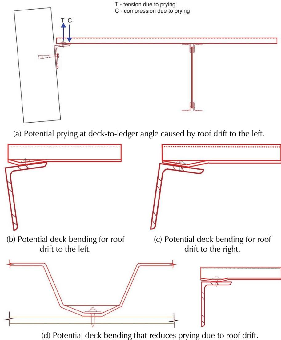
Figure 8-9 Illustration of deck local bending that may reduce prying forces.
