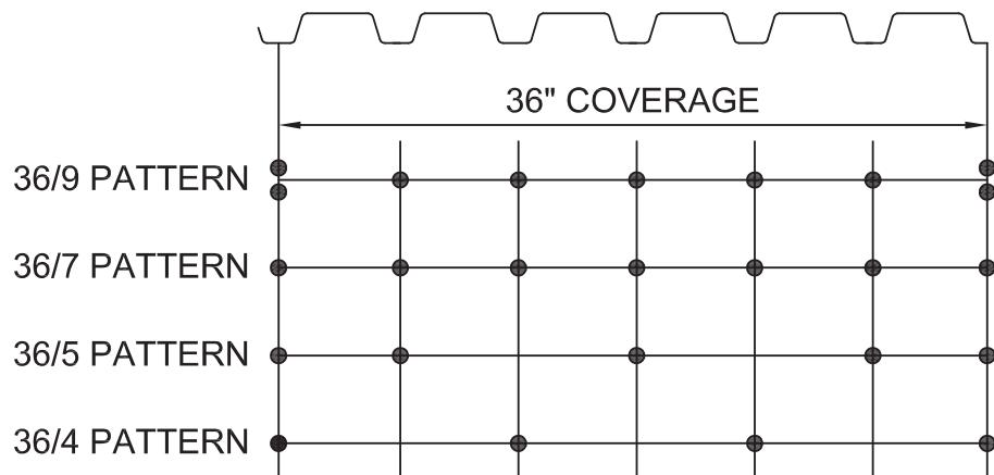
Figure 3-7 Typical fastener attachment patterns (see DDM04 for further details).
