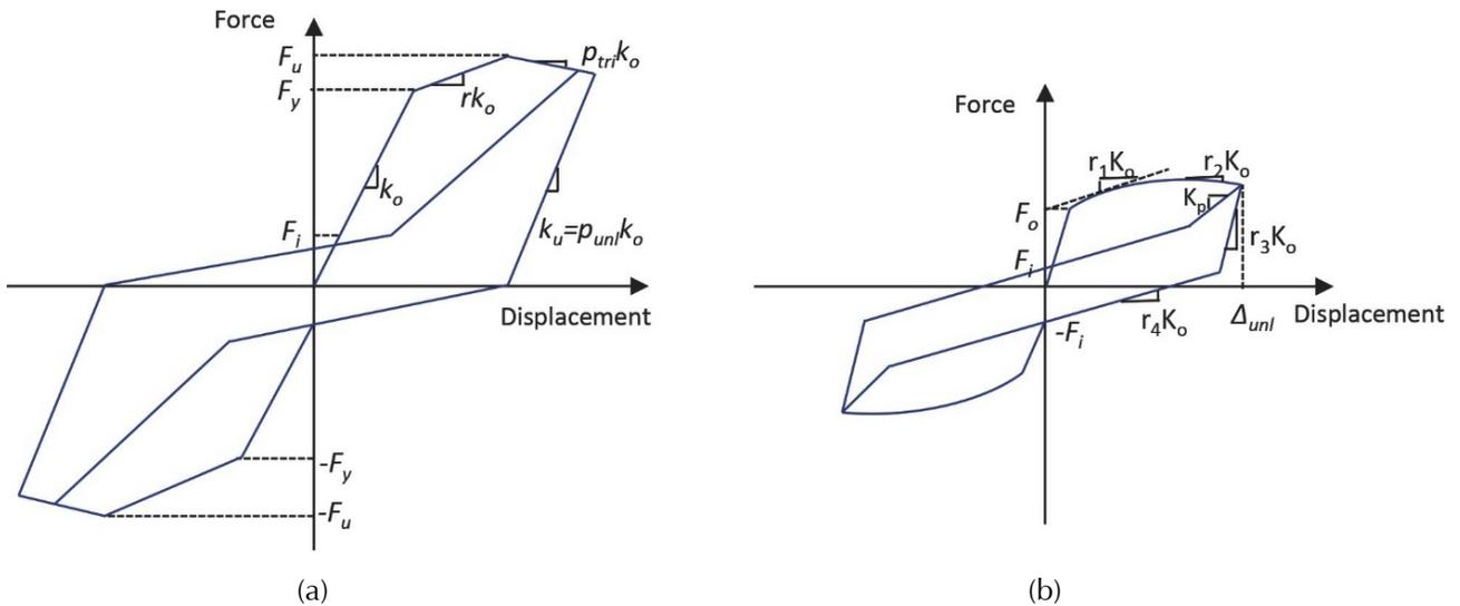
Figure A-2 Illustration of hysteretic models: (a) Wayne-Stewart; and (b) SAWS.
