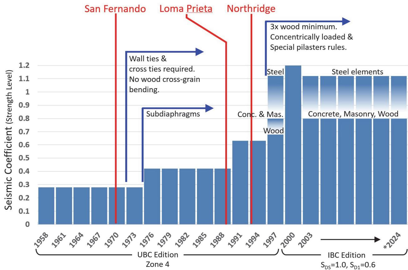
Figure 2-6 Evolution of wall anchorage code provisions (figure credit: Lawson et al., 2018 with update by Lawson, 2021).
