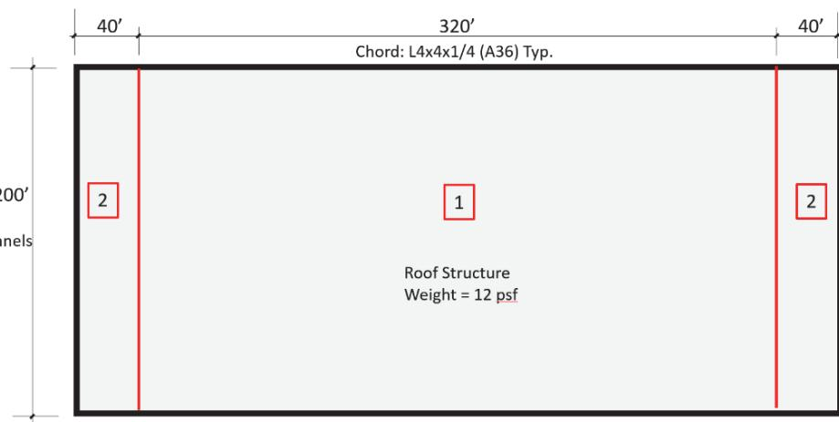
Figure C-6      Design details for archetypes with wood diaphragms designed for moderate-seismic hazard, part 1 (alternative RWFD procedure).
