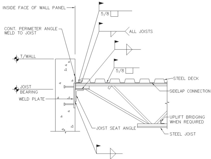
Figure 8-8 Example detail of joist seat supported by a seat angle (image credit: Joseph Steinbicker).
