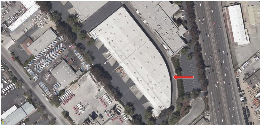
Figure 8-5 Example of a RWFD building with nonparallel walls (photo credit: ConnectExplorer).
