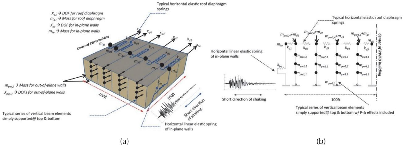
Figure A-6 Illustration of a simplified RWFD building model developed in the RUAUMOKO2D platform.
