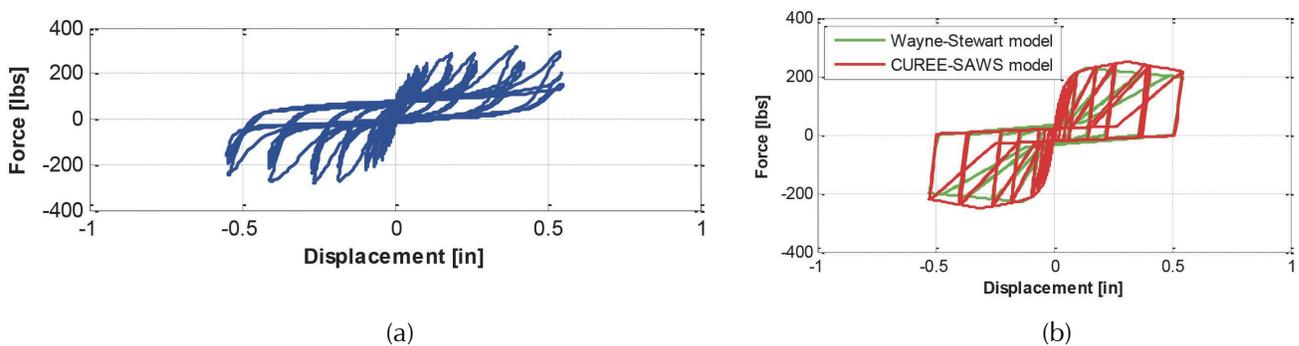
Figure A-3 Comparison of hysteretic response for 10d common nail and wood deck: (a) example of experimental data (Coyné, 2007) and (b) best fit numerical model based on data from several tests (Koliou, 2014).
