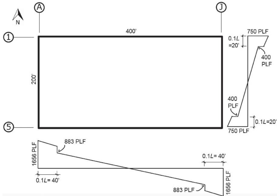
Figure 5-3 Shear diagrams for the diaphragm design with the 1.5 × factor.
