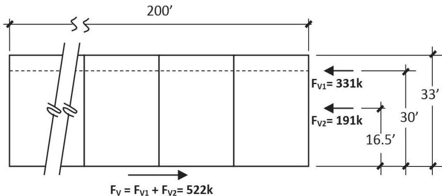
Figure 3-12 North/south lateral design forces acting on the shear walls (Lines A & J).
