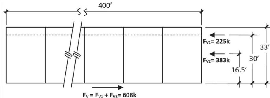
Figure 5-13 East/west lateral design forces acting on the shear walls (Lines 1 & 5) (repeated).
