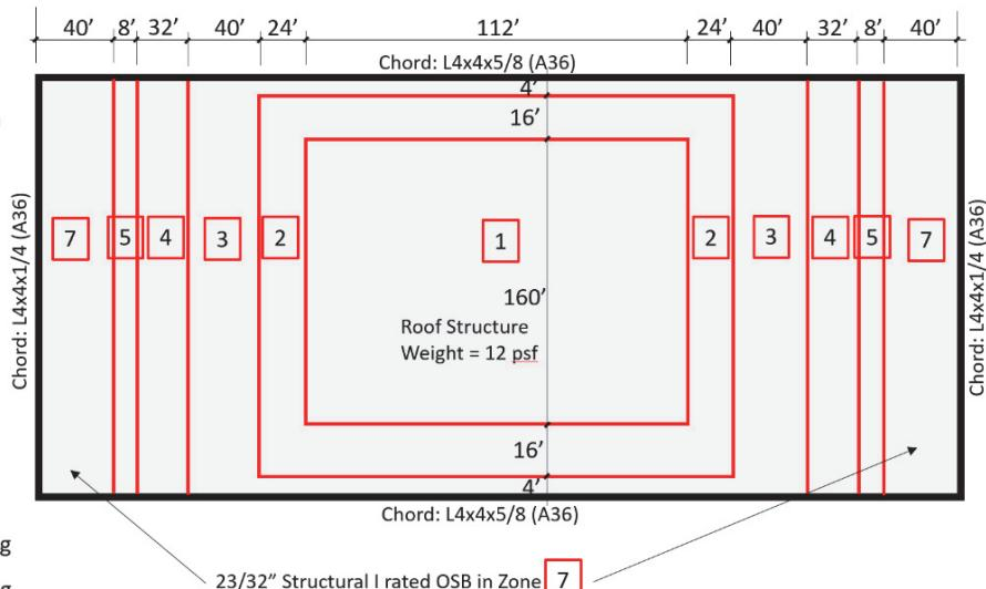
Figure C-3 Design details for archetypes with wood diaphragms designed for high-seismic hazard, part 3 (alternative RWFD procedure).
