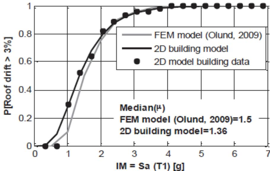
Figure A-9 Incremental dynamic analysis results/comparison.
