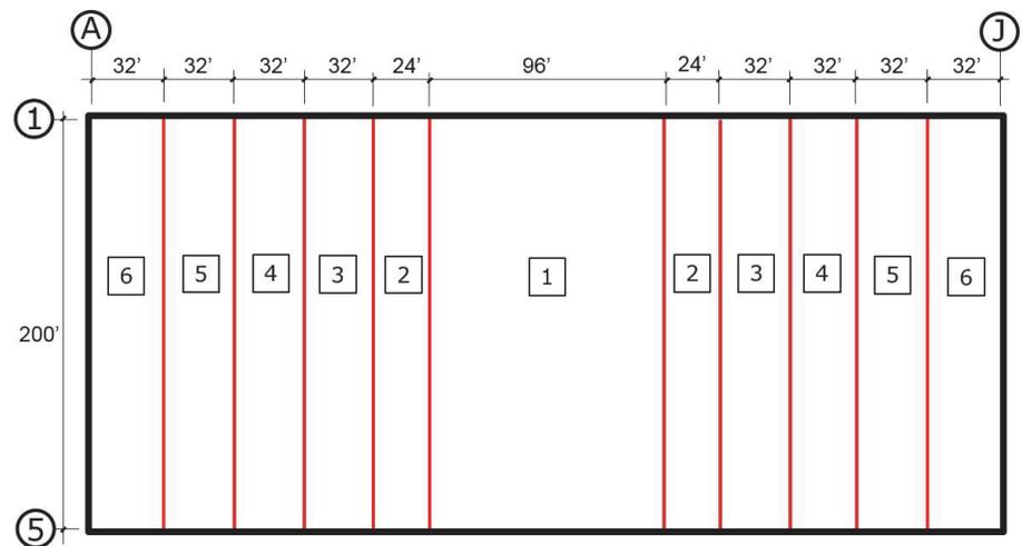
Figure 3-5 North/south nailing zone layout.
