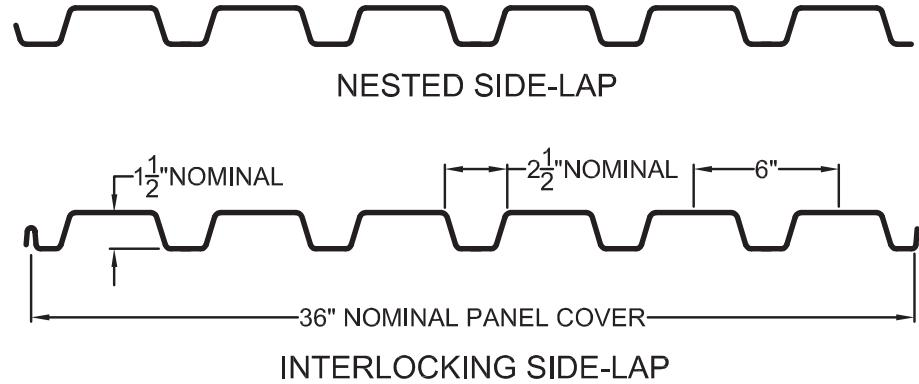
Figure 3-6 WR deck dimensions (see DDM04 for further details).
