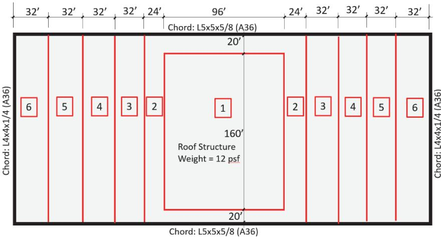
Figure B-2 Design details for the "large" archetypes with wood diaphragms designed for high-seismic hazard (traditional procedure).
