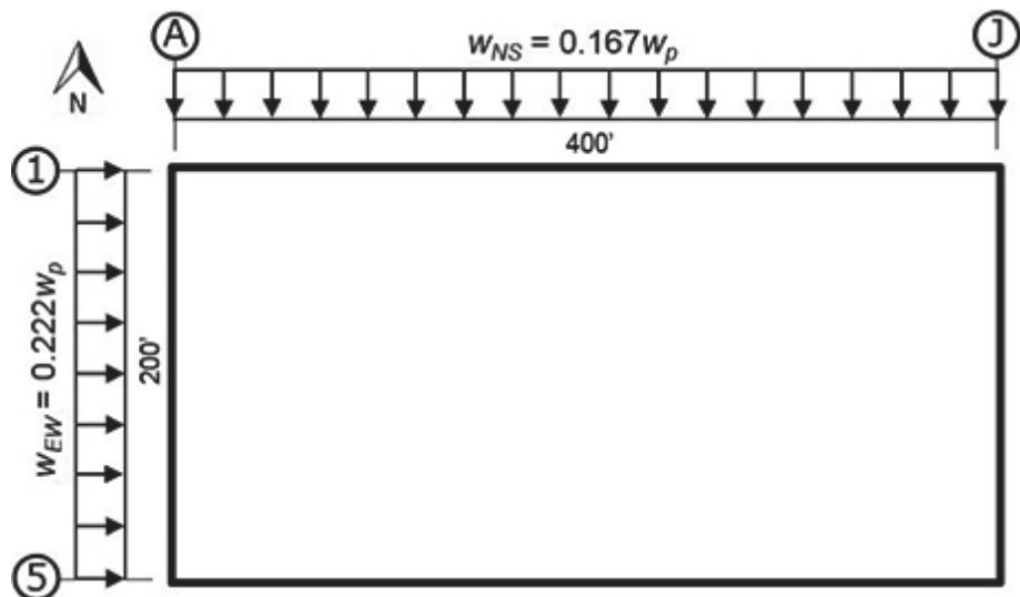
Figure 5-1 Diaphragm loading model (alternative RWFD procedure).
