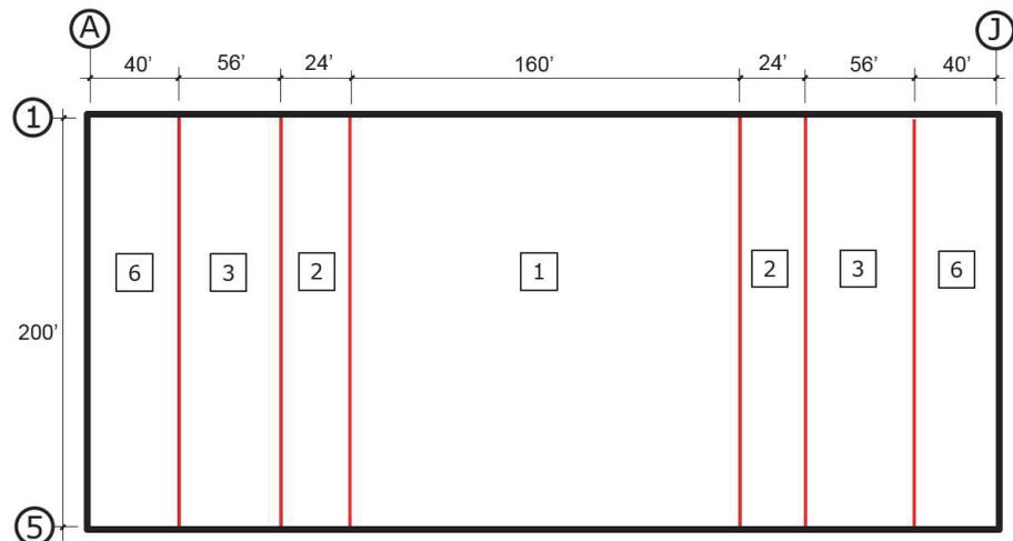
Figure 5-4 North/south nailing zone layout.
