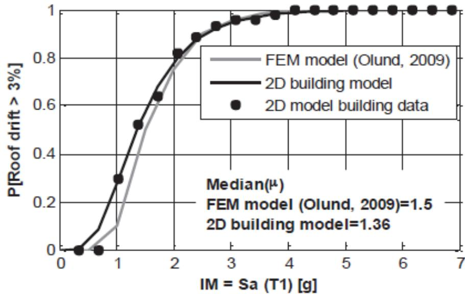
Figure A-9 Incremental dynamic analysis results/comparison.
