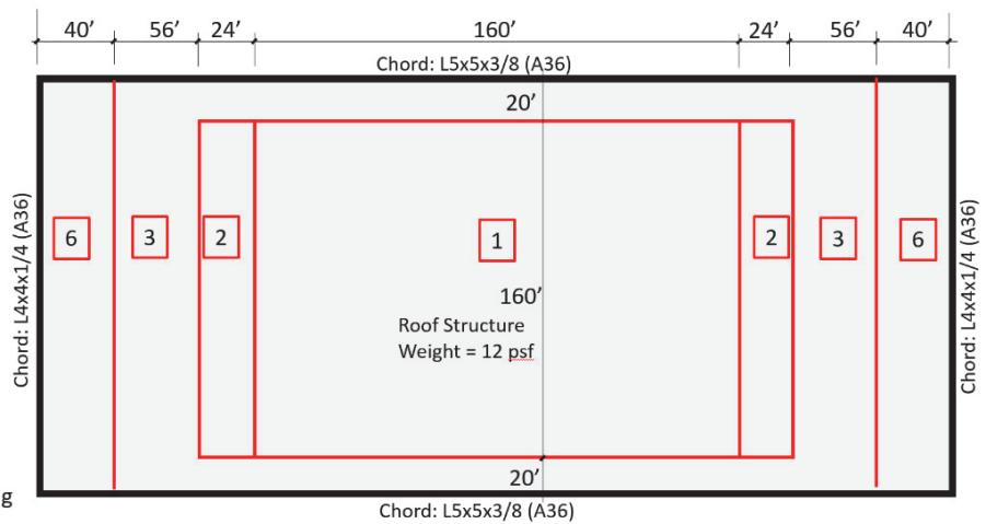
Figure C-2 Design details for archetypes with wood diaphragms designed for high-seismic hazard, part 2 (alternative RWFD procedure).
