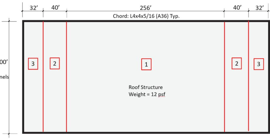
Figure B-4 Design details for "large" archetypes with wood diaphragms designed for moderate-seismic hazard (traditional procedure).
