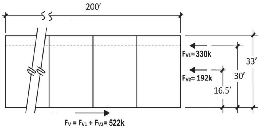
Figure 5-12 North/south lateral design forces acting on the shear walls (Lines A & J).
