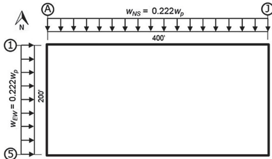
Figure 5-8 Diaphragm loading model (alternative RWFD procedure).
