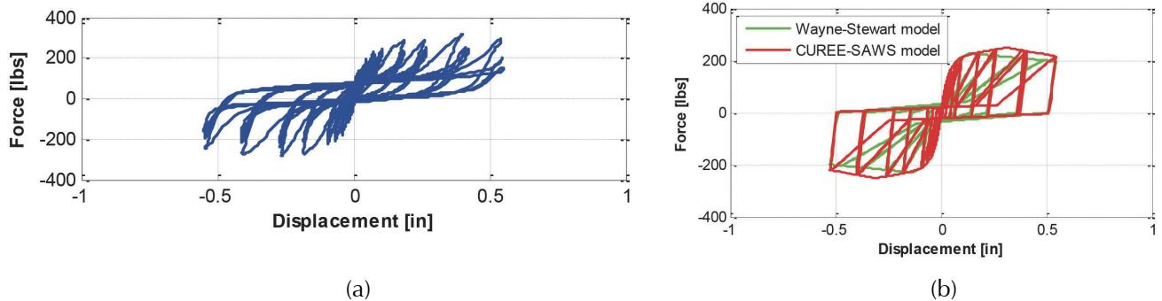
Figure A-3 Comparison of hysteretic response for 10d common nail and wood deck: (a) example of experimental data (Coyne, 2007) and (b) best fit numerical model based on data from several tests (Koliou, 2014).
