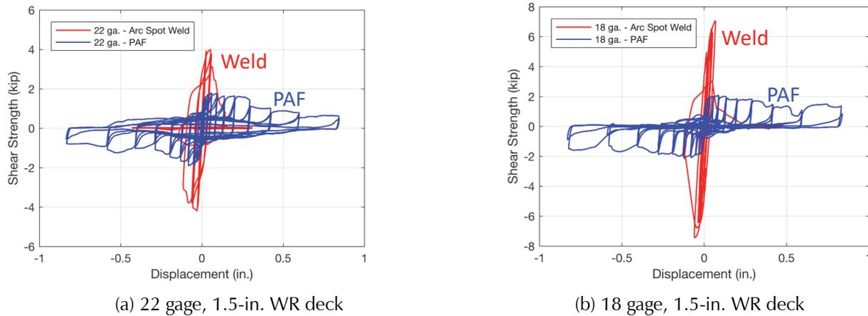
Figure D-2 Performance of PAF vs. arc-spot-weld structural connectors (image credit: Schafer, 2019 based on data in Torabian and Schafer, 2021).
