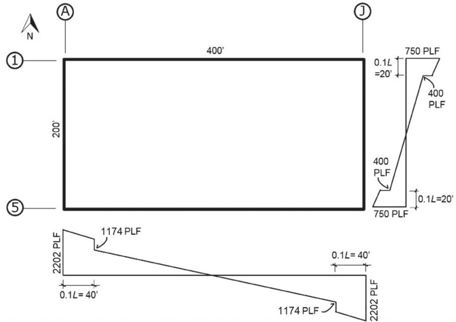
Figure 5-10 Shear diagrams for the diaphragm design with the 1.5× factor.
