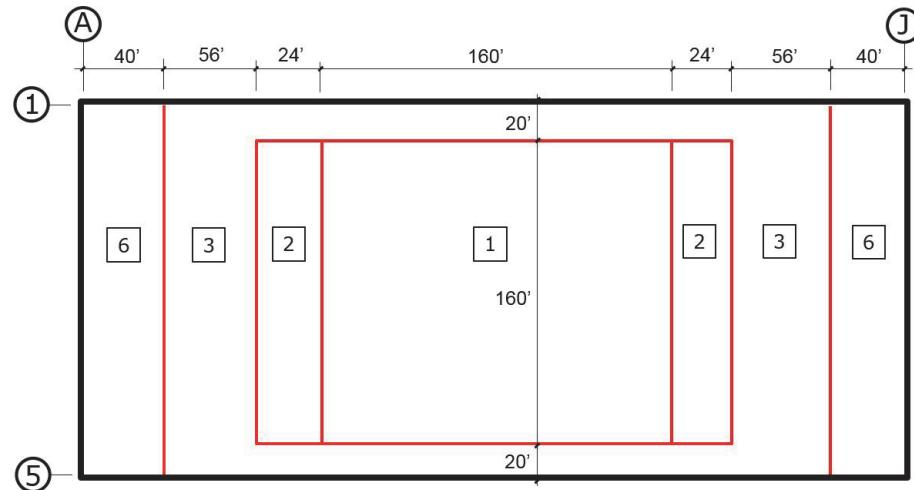
Figure 5-5 North/south and east/west nailing zones combined layout.
