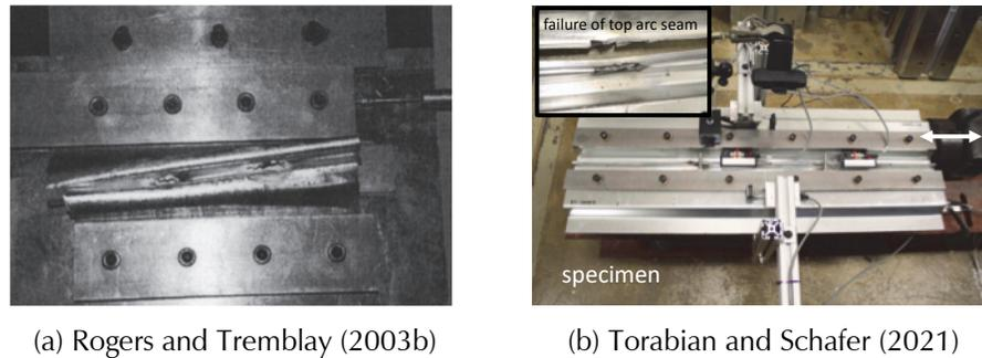
Figure D-1 Comparison of testing for top-arc seam weld as employed for connector data: (a) as used in Koliou (2014) based on Rogers and Tremblay (2003b), and (b) as used herein based on Torabian and Schafer (2021).
