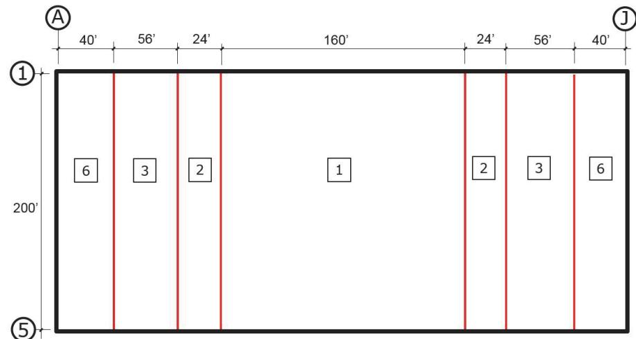
Figure 5-4 North/south nailing zone layout.
