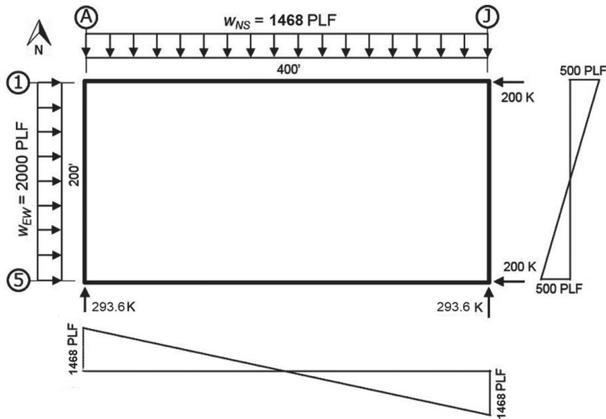
Figure 5-9 Diaphragm shear distribution.
