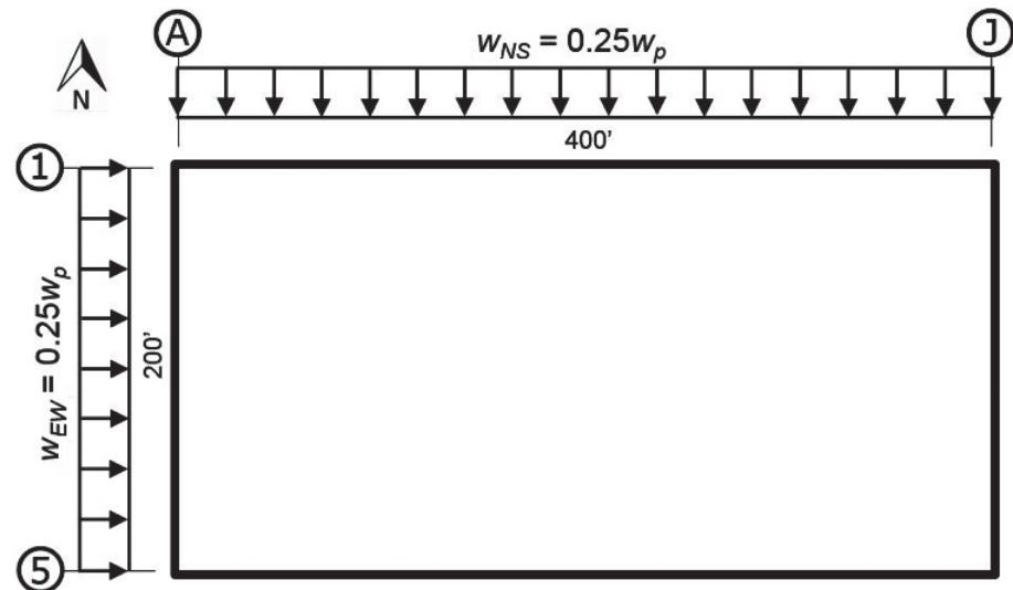
Figure 3-2 Diaphragm loading model (both orthogonal directions shown).
