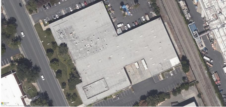
Figure 8-1 Example of a RWFD building with a large re-entrant corner (photo credit: ConnectExplorer).
