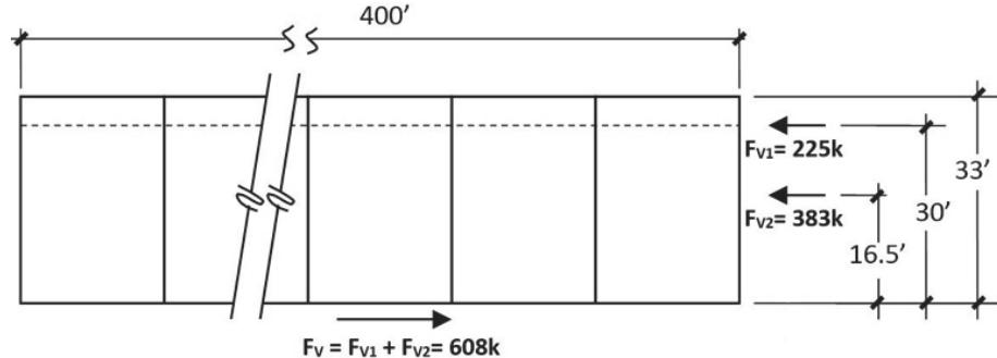
Figure 3-13 East/west lateral design forces acting on the shear walls (Lines 1 & 5).
