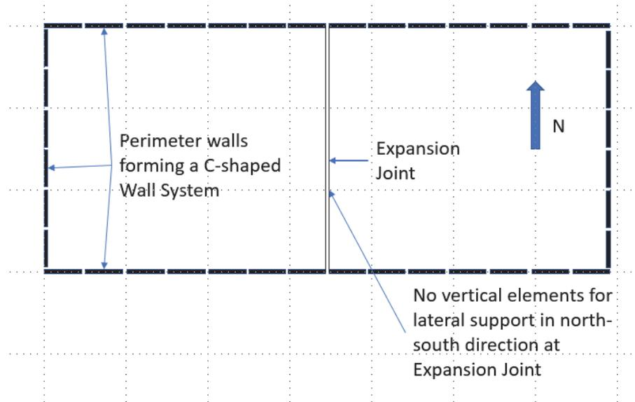
Figure 8-6 C-shaped lateral-system configuration.
