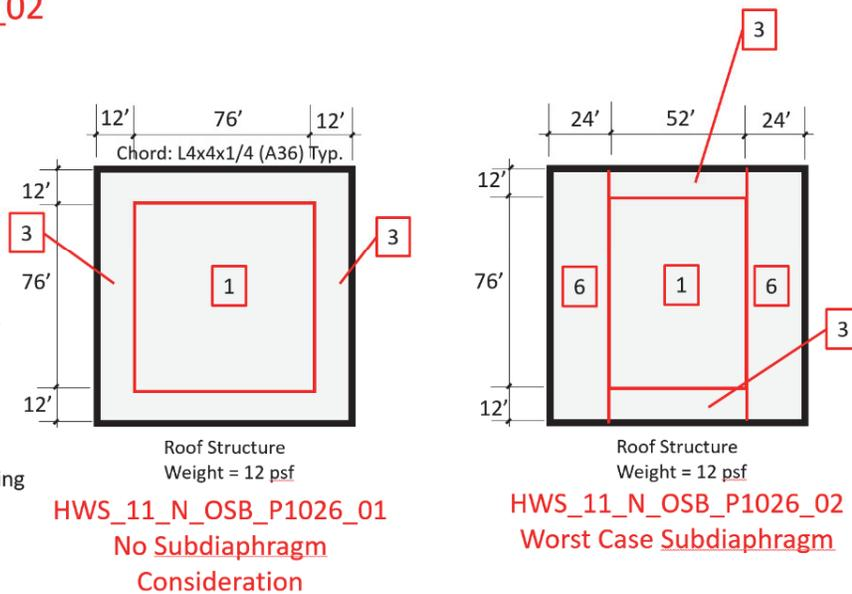
Figure C-5 Design details for archetypes with wood diaphragms designed for high-seismic hazard, part 5 (alternative RWFD procedure).
