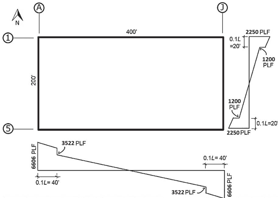
Figure 5-14 Shear diagrams for the diaphragm design with the 1.5x factor in the base of a steel deck roof that does not meet special seismic detailing.
