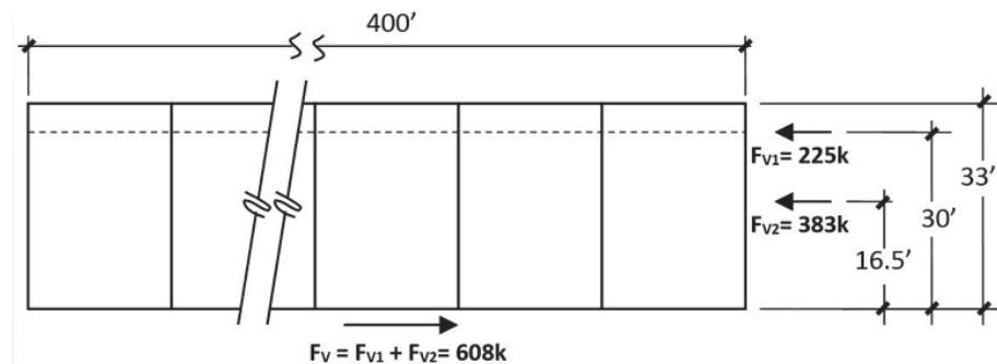
Figure 5-7      East/west lateral design forces acting on the shear walls (Lines 1 & 5).
