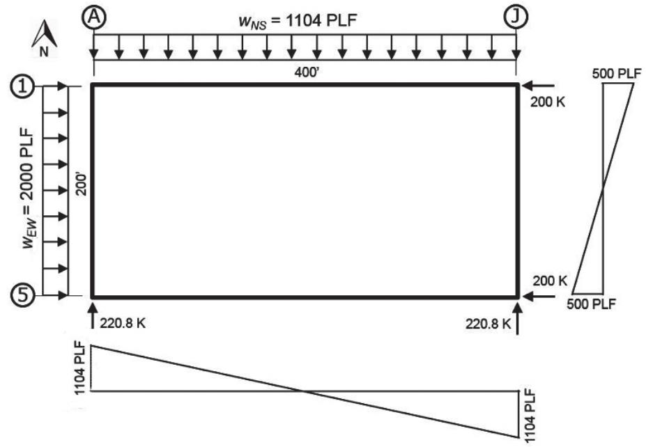
Figure 5-2 Diaphragm shear distribution.
