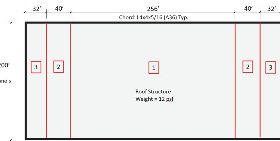
Figure B-4 Design details for “large” archetypes with wood diaphragms designed for moderate-seismic hazard (traditional procedure).
