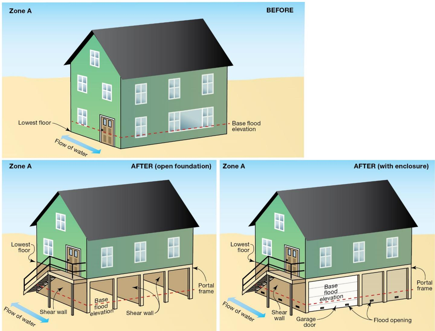
Note: Drawing is not to scale. The number of flood openings shown is for illustration purposes only; the total number of openings depends on the square footage of the enclosure and the type and design of the opening.
