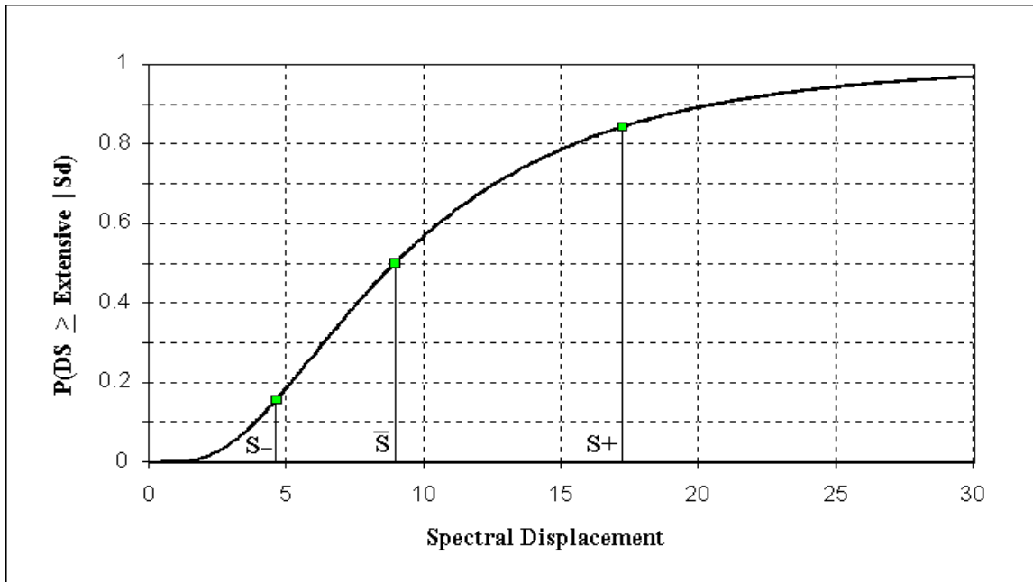
Figure 5.5 Example Fragility Curve - Extensive Structural Damage, C1M Model Building Type, High-Code Seismic Design.
