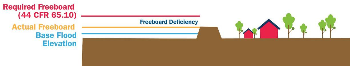
*The yellow line shows the height of the levee. While it is above the BFE, it does not meet the red line, which is the required freeboard the levee would need to meet 65.10.*
