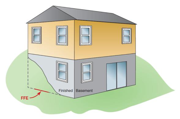
Figure 2.9: FFE for a finished walkout basement
