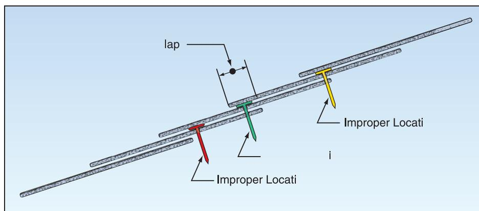
**Figure 11-36.** Proper and improper location of shingle fasteners (nails). When properly located, the nail engages the underlying shingle in the headlap area (center nail). When too high, the nail misses the underlying shingle (left nail) or is too close to the edge of the underlying shingle (right nail)
