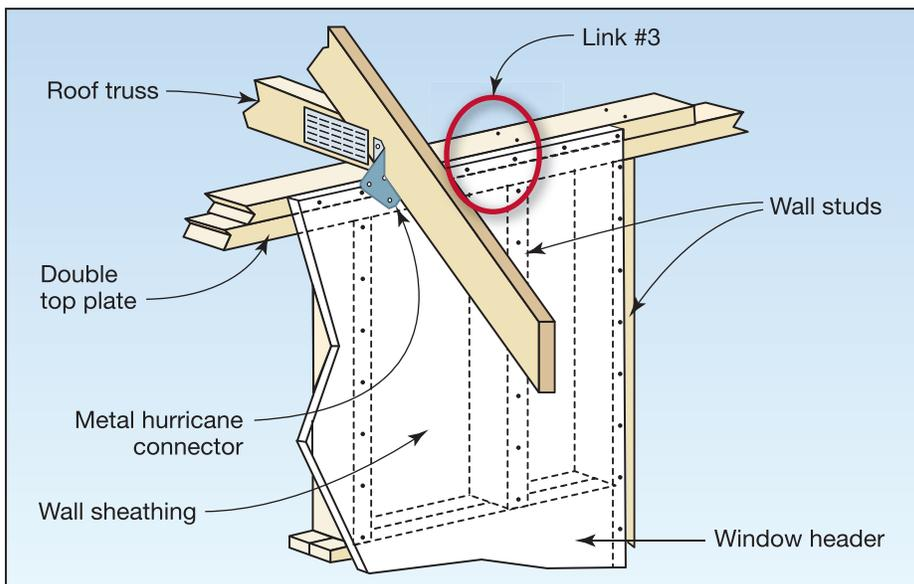
**Figure 9-11.** Connection of wall top plate-to-wall stud (Link #3)
