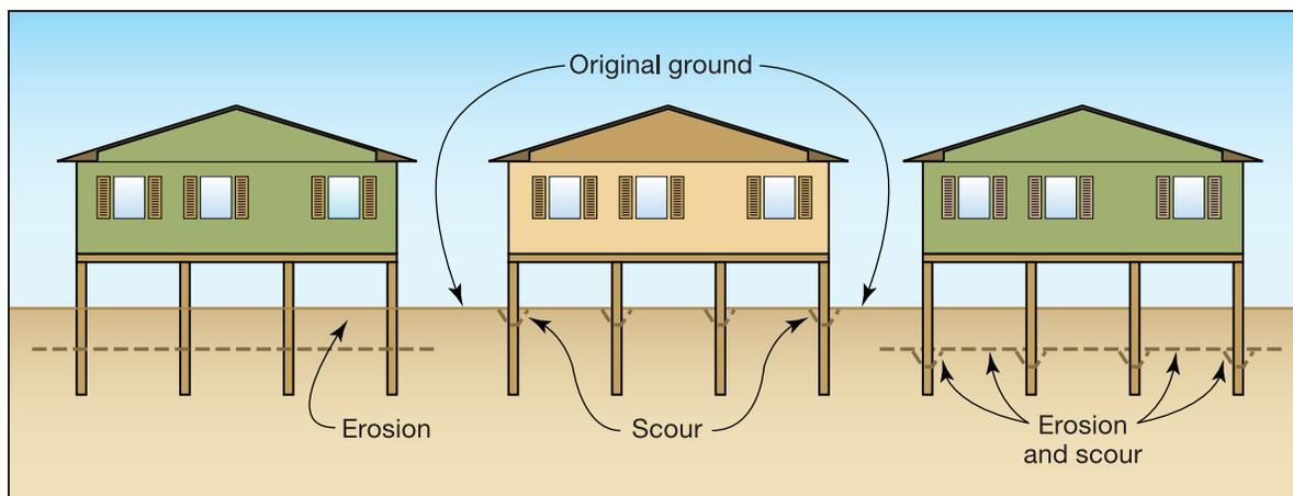
Figure 10-6. Scour and erosion effects on piling embedment
