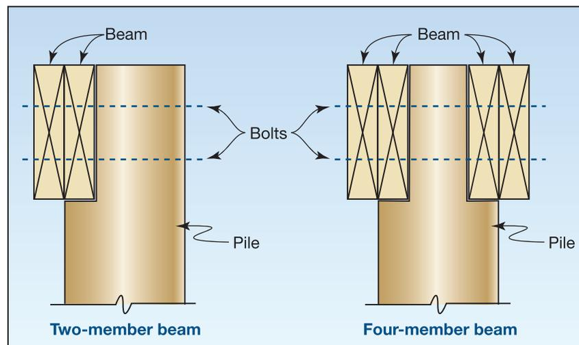
illustrates the proper pile notching for both two-member and four-member beams. See Section 13.1.1 for more information on pile notching.
