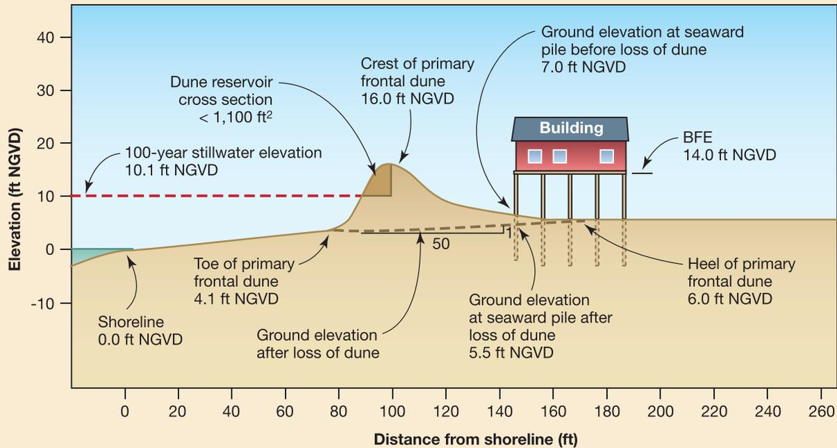
Illustration B. Primary frontal dune will be lost to erosion during a 100-year flood because dune reservoir is less than 1,100 ft<sup>2</sup> (Section A of Illustration A)
