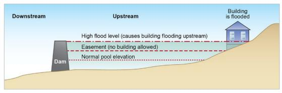
Figure 1: Upstream flooding increases pool elevations beyond easements
