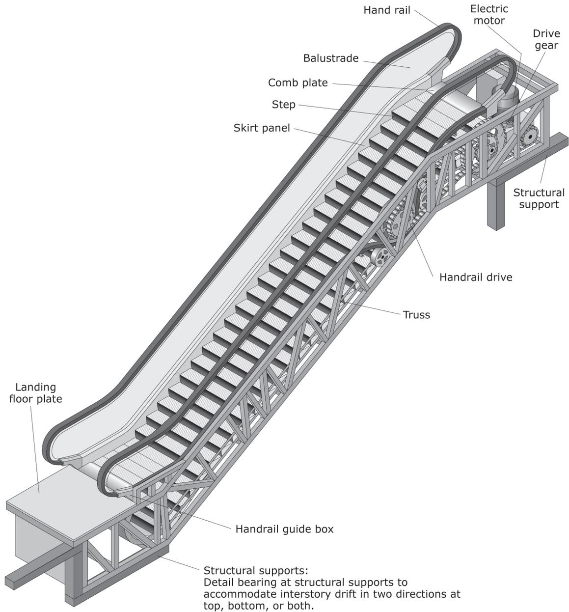
Figure 5-26. Typical elements of an escalator (Source: Otis Elevator Company).
