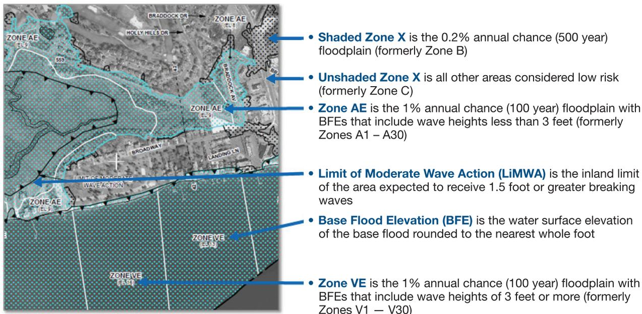
Figure 1-3. Conceptual FIRM showing representative coastal flood zones.
