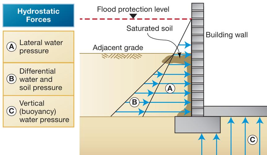
Figure 1-4. Hydrostatic forces.
