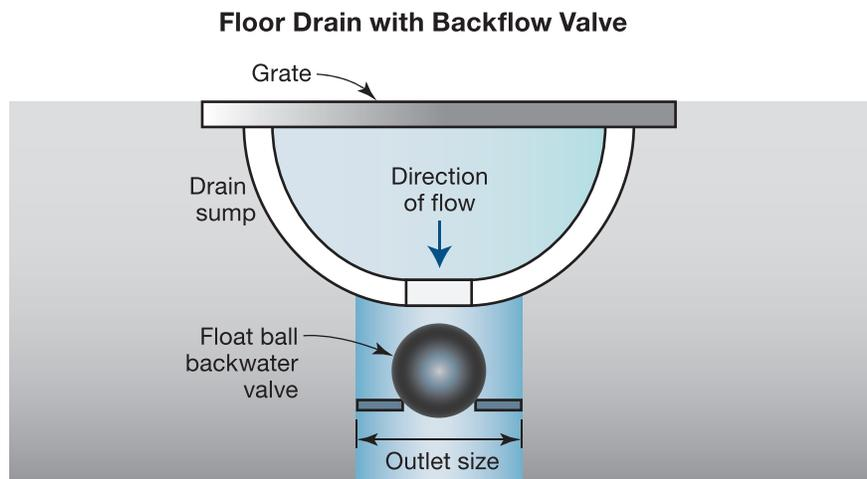
Although manually operated valves are available, it is recommended that homeowners consider automatic valves. Backflow through sewage pipes may result from a backup some distance away from the house and occur with little or no notice, so manual valves may not be as convenient. Manual valves can be installed to augment automatic valves, but if they are used, manually operated backflow valves should be closed well before flooding is expected.
