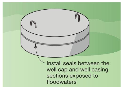
Figure 4-26. Concrete well cap and the uppermost section of concrete casing.
