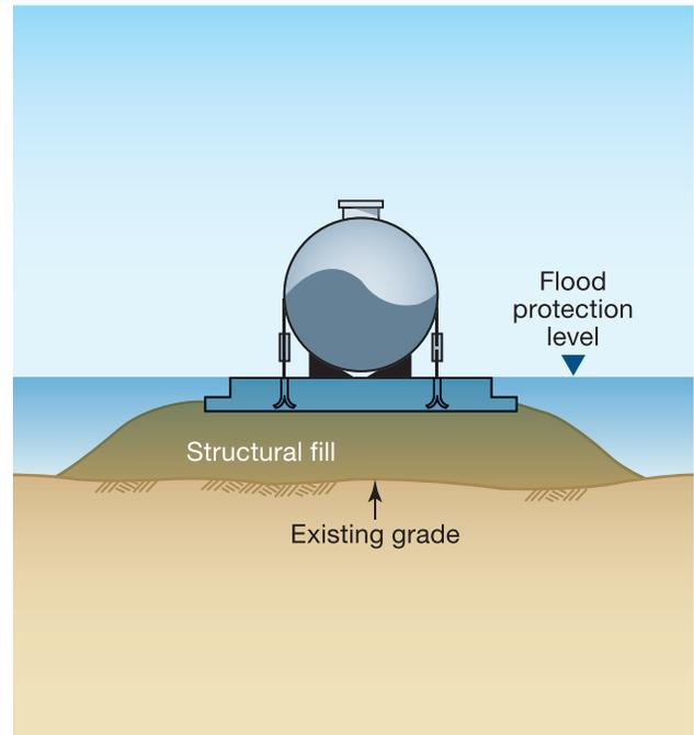
Figure 4-33. Fuel tank elevated on structural fill.
