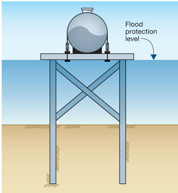
Figure 4-32. Fuel tank elevated on a supporting frame.
