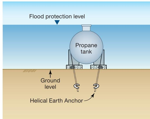
Figure 4-35. Above-ground tank secured with helical earth anchors.
