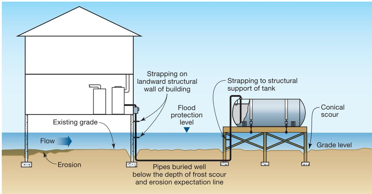
Figure 4-31. Protecting fuel piping from moving floodwater.
