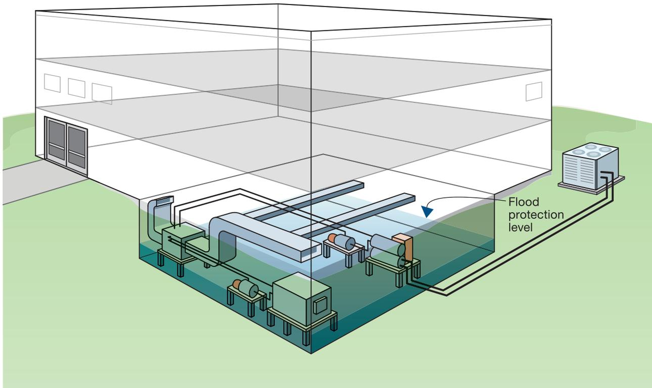
**Figure 5-8. In-Place Equipment Elevation of primary HVAC components elevated on supports or frames. Note the source of the flooding in the basement areas can greatly impact the effectiveness of flood protection measures.**
