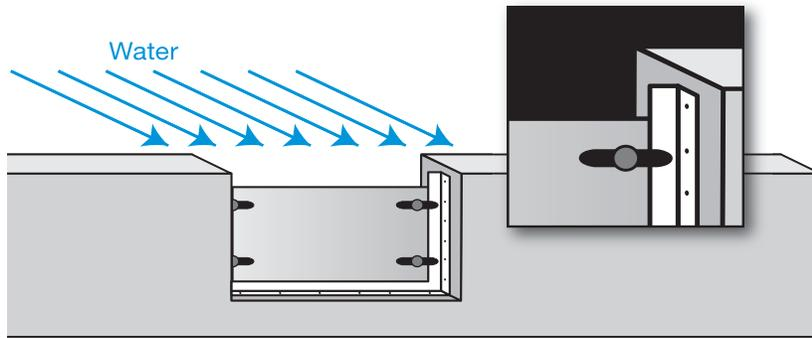
Latching dogs are commonly used to secure a closure panel
