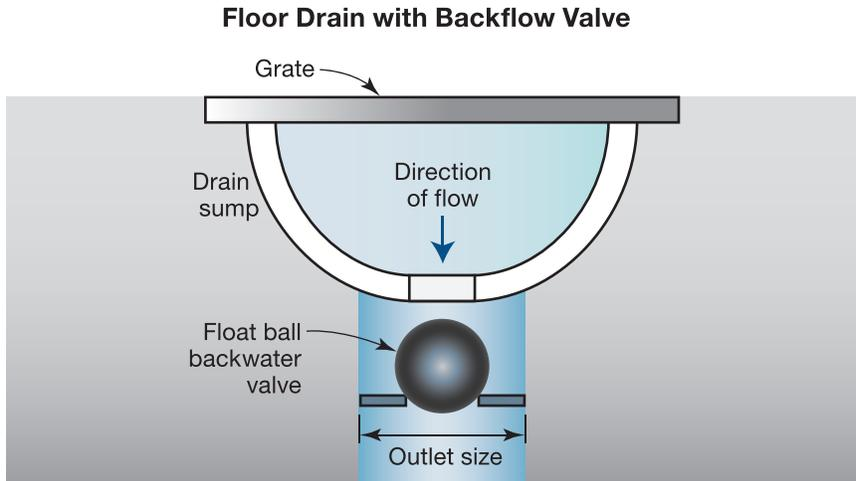
Figure 5-19. Floor drain with ball float check valve.
