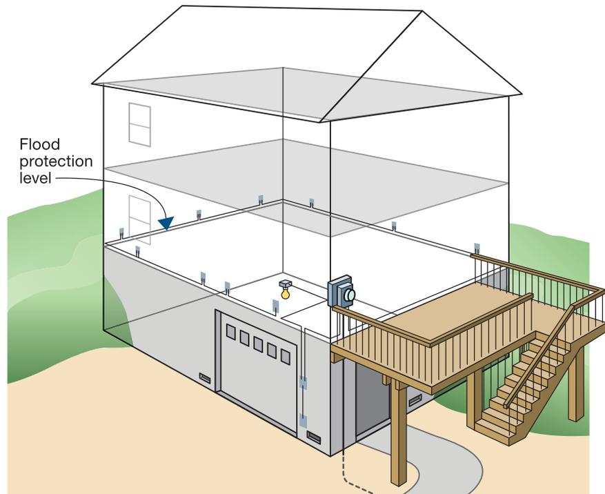
**Component Protection (Dry floodproofing):** Dry floodproofing can be considered as an interim mitigation option for electrical system components in existing homes that are not Substantially Improved. Dry floodproofing will not lead to full compliance with building codes, standards or the NFIP.
