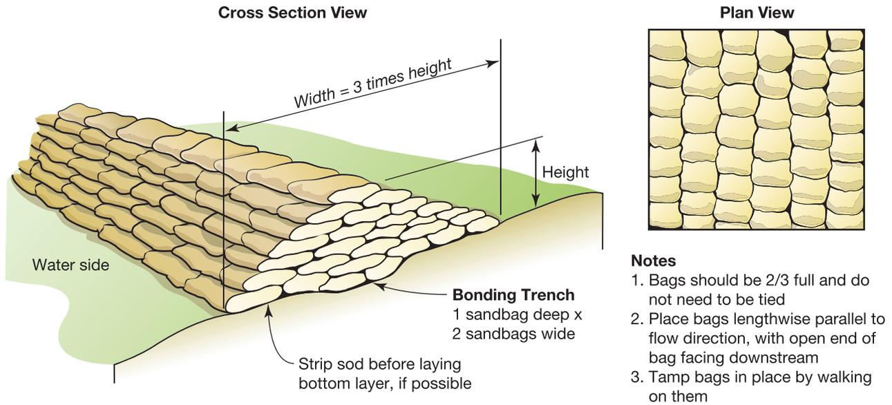
Figure 3-5. Techniques for proper placement of sandbags.
