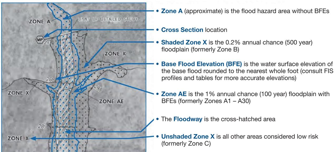
Figure 1-2. Conceptual FIRM showing representative riverine flood zones.
