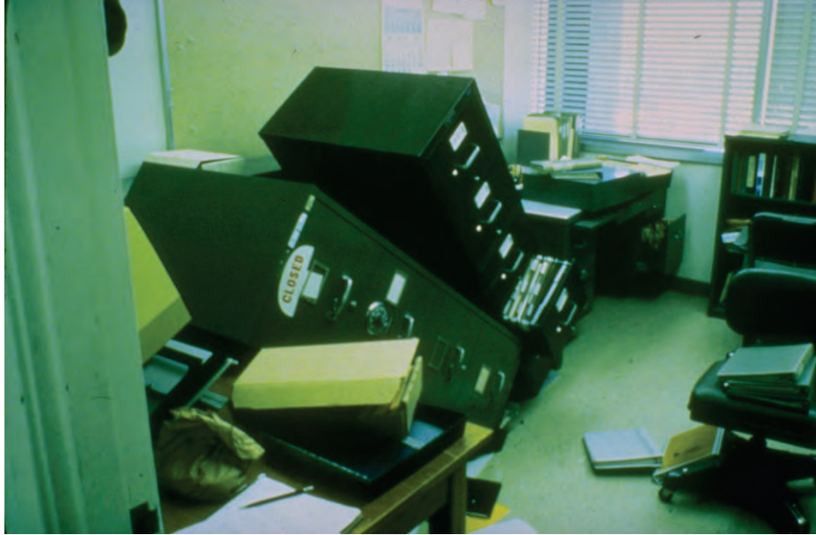
Figure 6.5.5.1-2 Tipped filing cabinets and other office equipment at the Lawrence Livermore Lab, California (NGDC, 2009).
