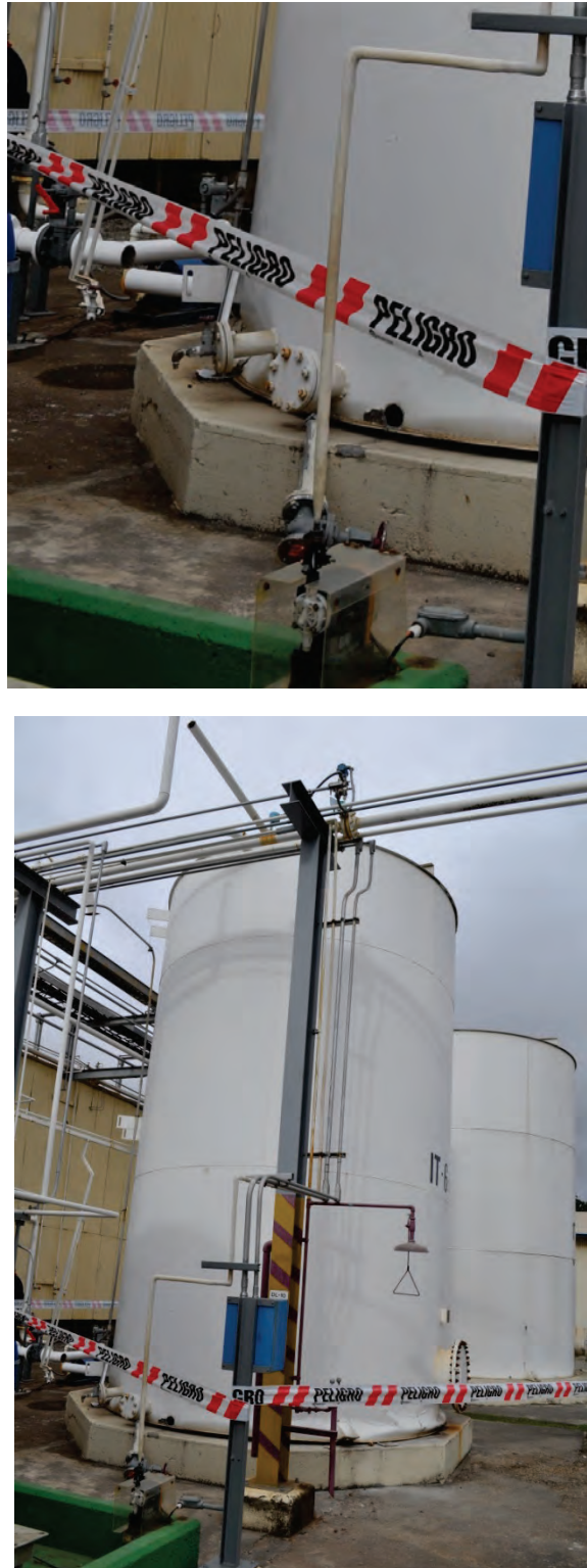
Figure 6.4.5.1-3 Elephant foot damage to inadequately anchored fuel tank in the 2010 Chile Earthquake also resulted in damage to fuel lines. Close-up photo shows failed pipe at welded joint (left) and pipe segment with attached valve (foreground) tore out of the tank wall (Photos courtesy of Eduardo Fierro, BFP Engineers).
