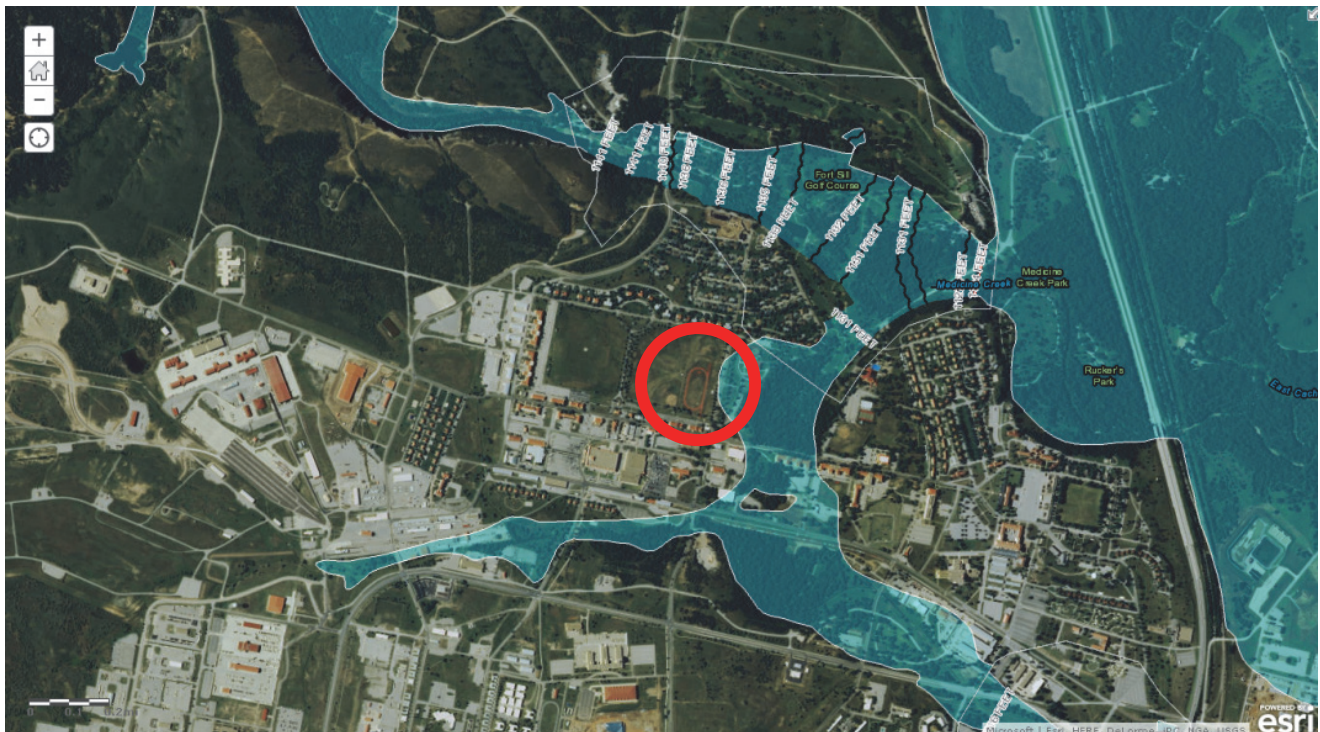
Figure AF-7 Portion of screenshot from the National Flood Hazard Layer for Lawton, Oklahoma. For comparison with Figure AF-8, the red circle is at a running track at Pritchard Field, outside the area expected to flood during the 1% annual chance flood – cyan shading).
