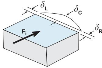
Figure 41 Deflection of diaphragm under lateral loading.
