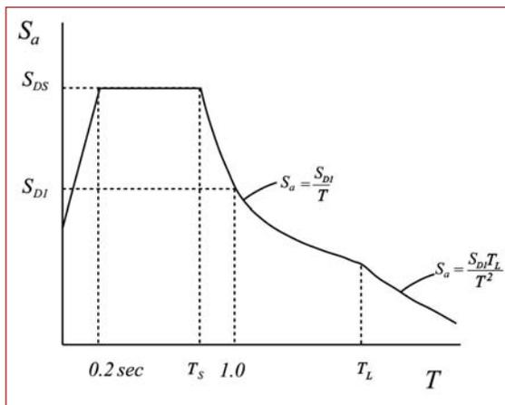
Figure 30 Generalized design response spectrum.
