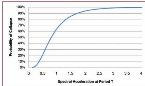
Figure 13 Collapse fragility curve for a hypothetical structure.
