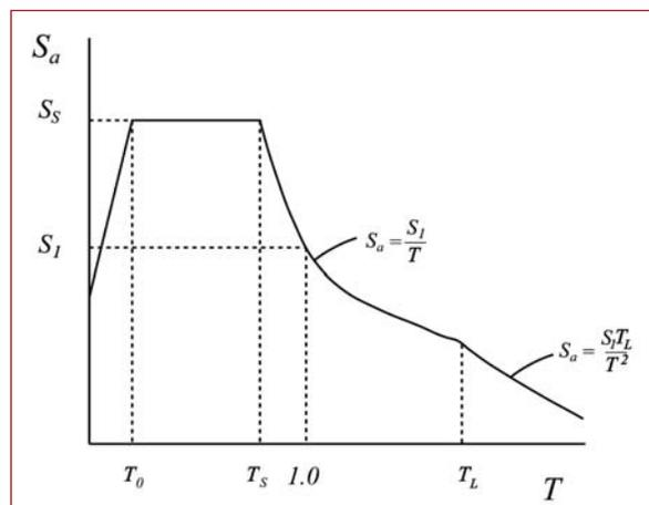
Figure 10 Generalized shape of smoothed response spectrum.
