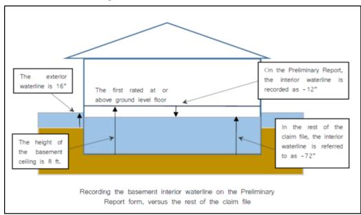
Figure 34: Basement Interior Waterline
