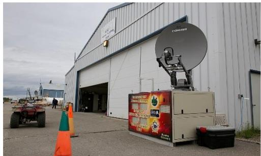
*In remote areas where cell phone and internet communication is sparse the Rapid Communication Ultra High Frequency satellite receiver is a key tool for emergency managers to operate recovery efforts.*
