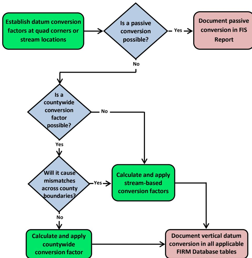
Figure 2: Detailed Vertical Datum Conversion Decision Process
