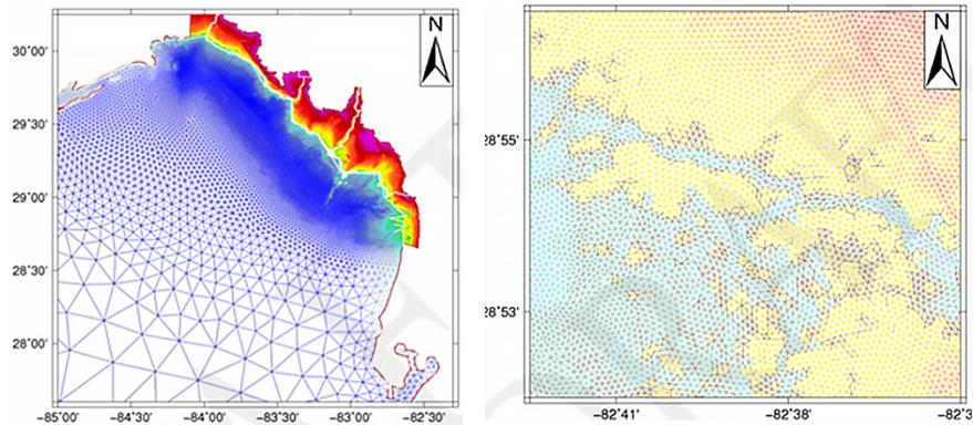
Figure 11. ADCIRC+SWAN Unstructured Mesh in the Big Bend Area
