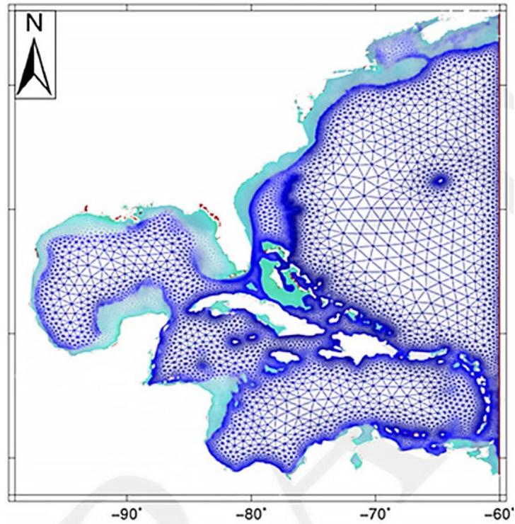
Figure 10. ADCIRC+SWAN Unstructured Mesh
