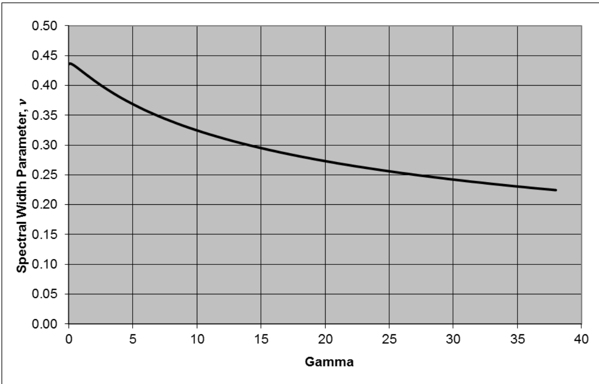
Figure 3-5. Spectral Width Parameter Versus Gamma for JONSWAP Spectra
