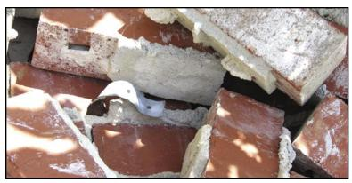
Figure 3. This tie remained embedded in the mortar joint while the smooth-shank nail pulled from the stud.
