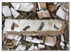
Figure 6. There were several ties in this portion of the wall, but they failed due to severe corrosion.
