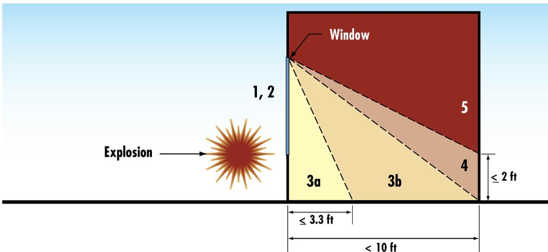
Figure 3-4 Side view of a test structure illustrating performance conditions of Table 3-2
