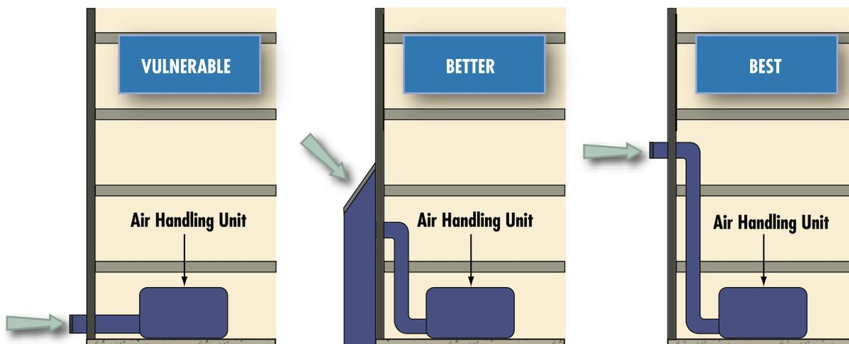
Figure 3-7 Example of protecting outdoor air intakes
