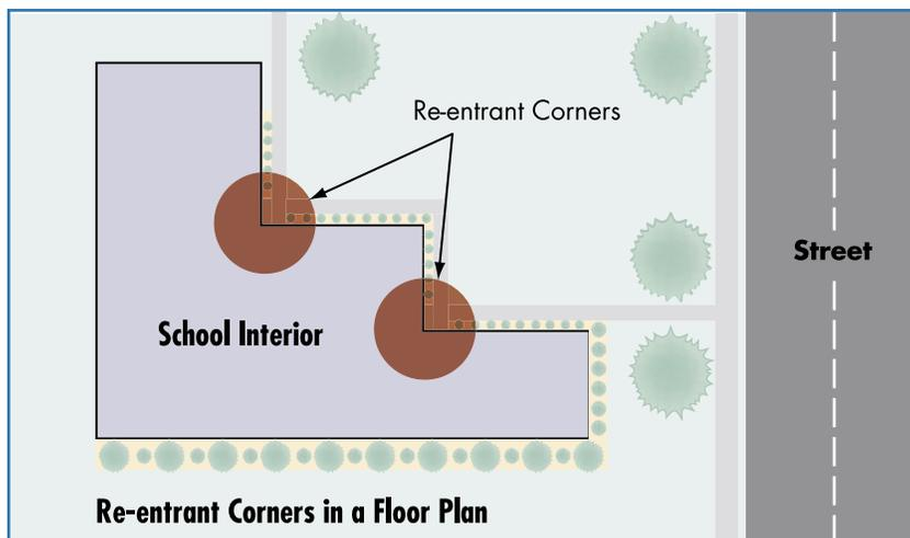
Figure 3-1 Re-entrant corners in a floor plan
