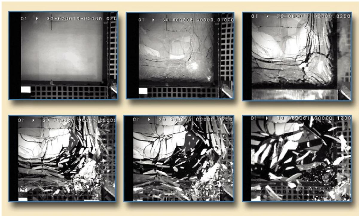
Figure 3-5 An unprotected window after a large explosion
