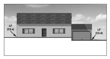
Letters and numbers in parentheses, as "(A8.c)" or "(C2.a)," correspond to Section A or Section C of the Elevation Certificate.
