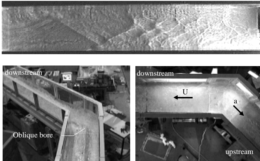
Fig. 1 Shock waves generated from 'dambreak' flow around a 45° bend.
