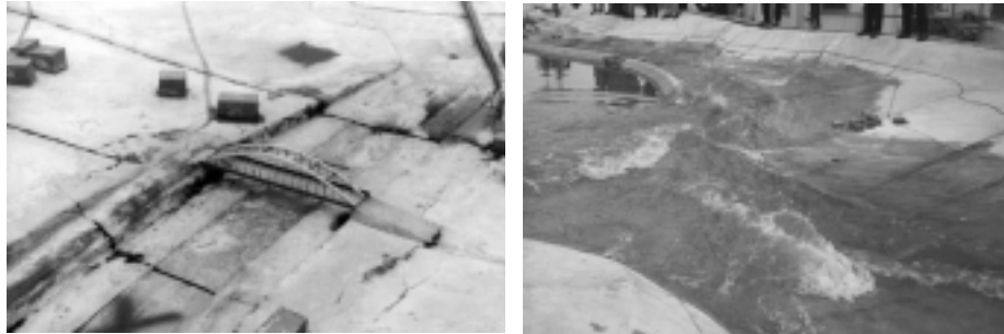
Photos courtesy of Prof JM Hiver, Université Libre de Bruxelles, Belgium Fig. 3 Bridge structure on the Toce model and a dambreak flow simulation
